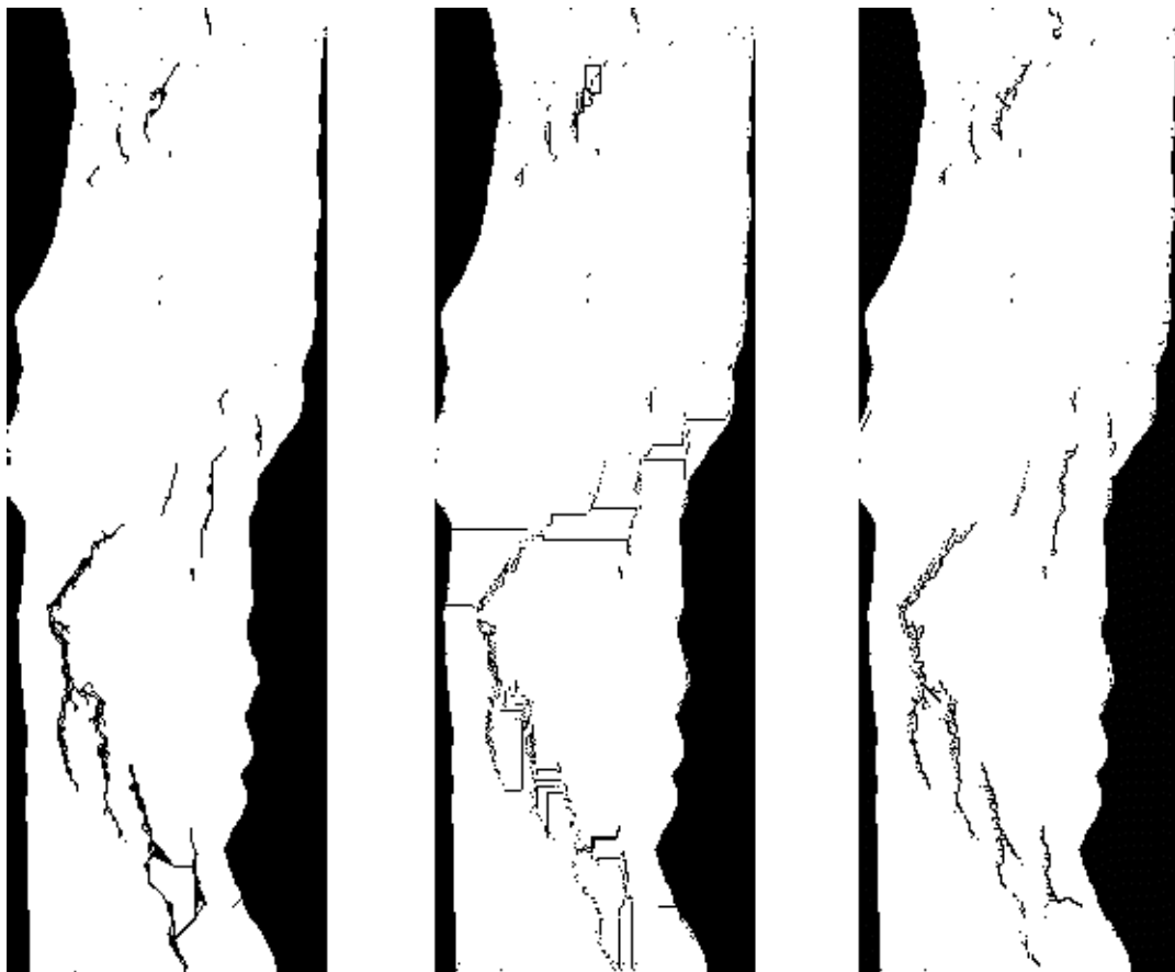
Figure 3. Branch cut images from different phase unwrapping algorithms. Left: The classical Goldstein algorithm shows one part completely isolated by branch cuts which leads to an incorrect unwrapping result. Centre: Branch cuts from MCF network with constant costs also show some erroneous connections. Right: Branch cuts from MCF network with costs derived from enhanced coherence values pass the visual inspection.
