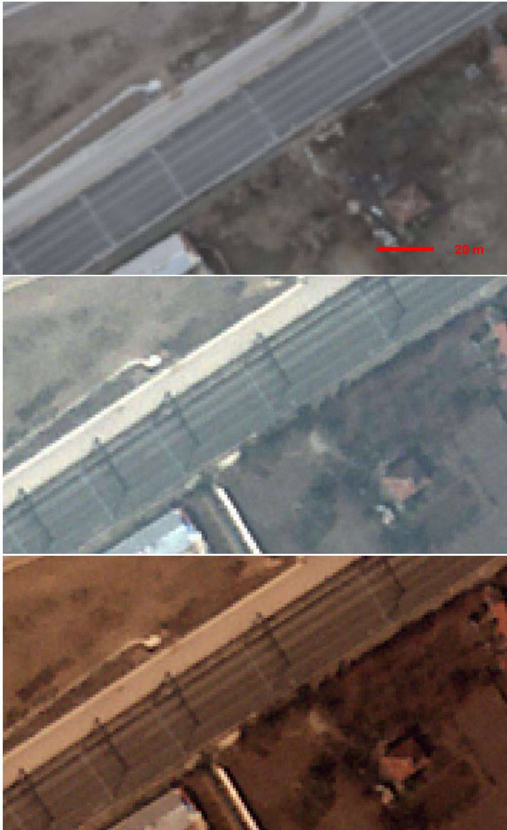
Figure 4-4: Comparisons with the UAV orthophoto over railways visible in: Top: UAV orthophoto; Middle: SN30 L1 image; Bottom: SN30 L3 image.
