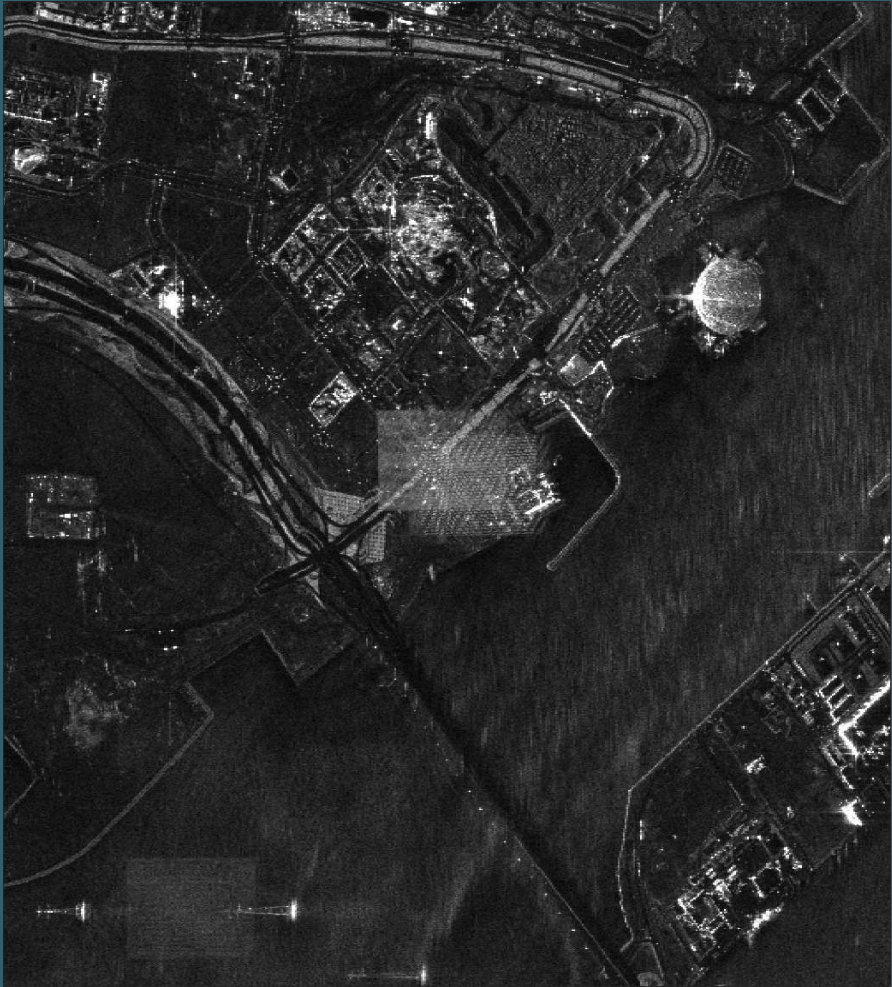
The ambiguities were generated by the secondary lobes of the azimuth antenna pattern
