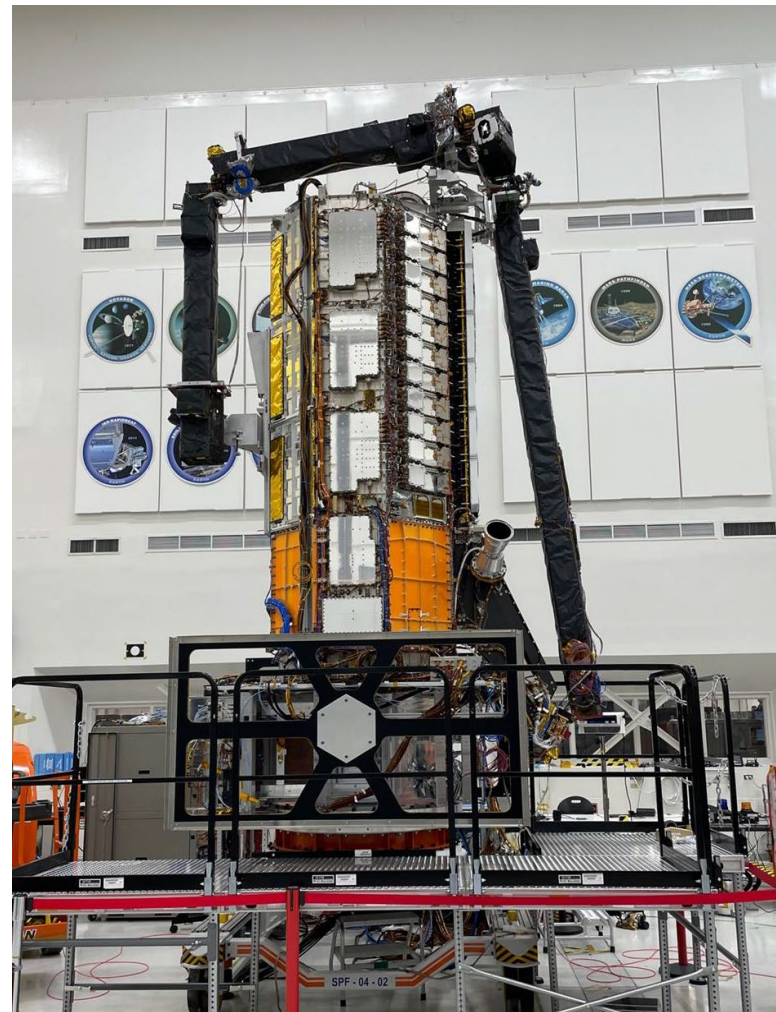
Flight Boom currently being integrated with flight model radar structure; Flight Reflector integration late May 2022
