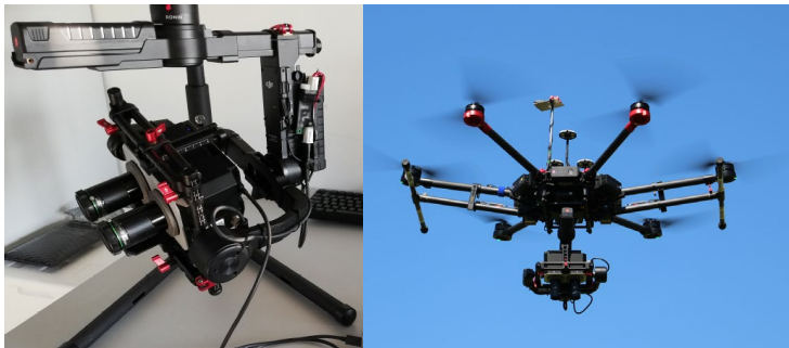
UAV Dual-camera system
