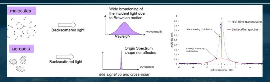
Brownian motion of molecules induces broadening of incident spectrum, whereas scattering with aerosol particles does not:
