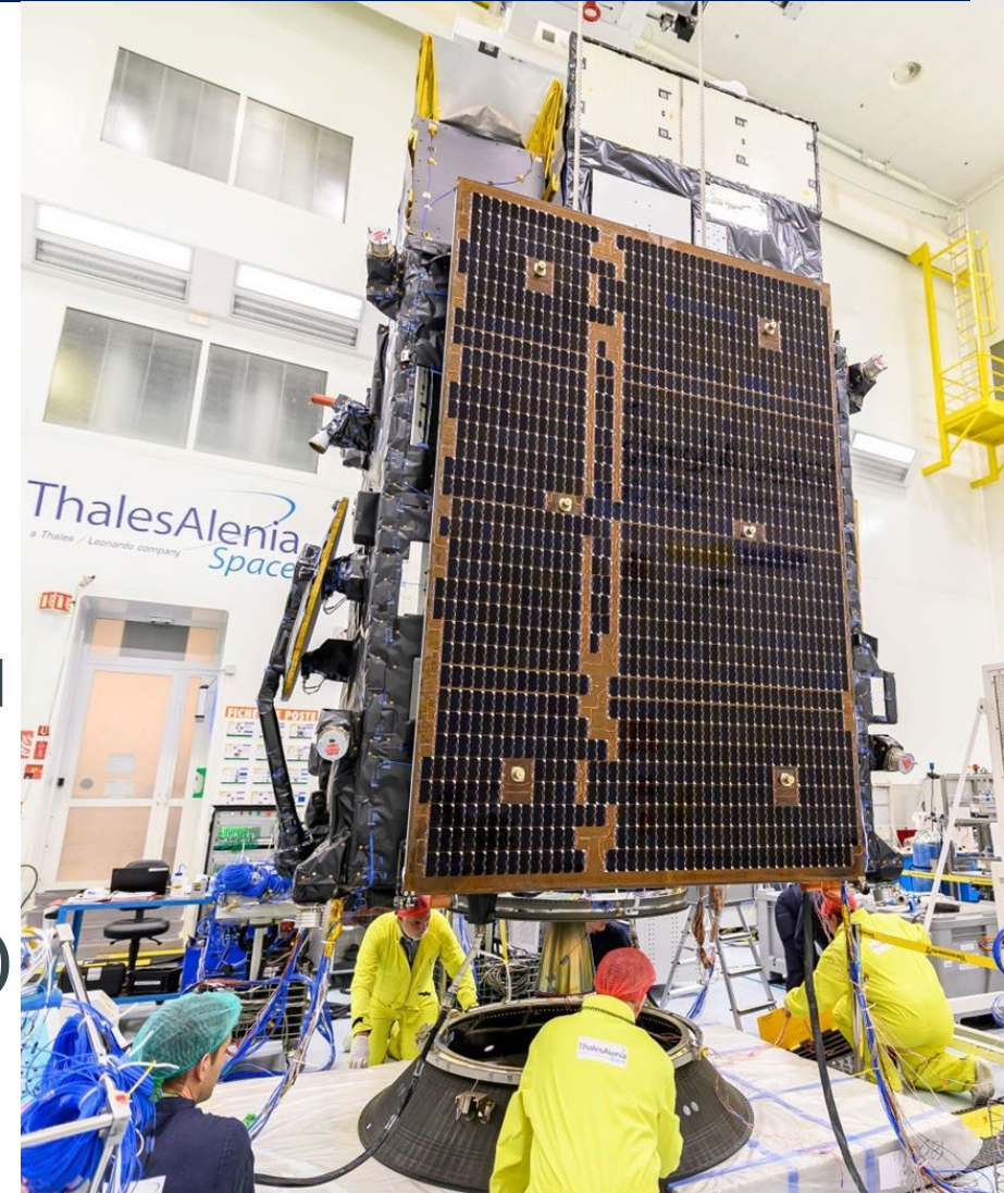
Complete MTG-I PFM satellite and its launch adapter after separation test (picture by Thales Alenia Space)
