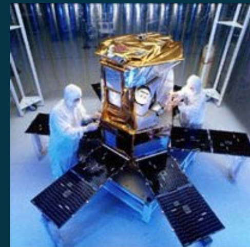
SORCE is 290 kg based on an Orbital LEOStar-2 bus
