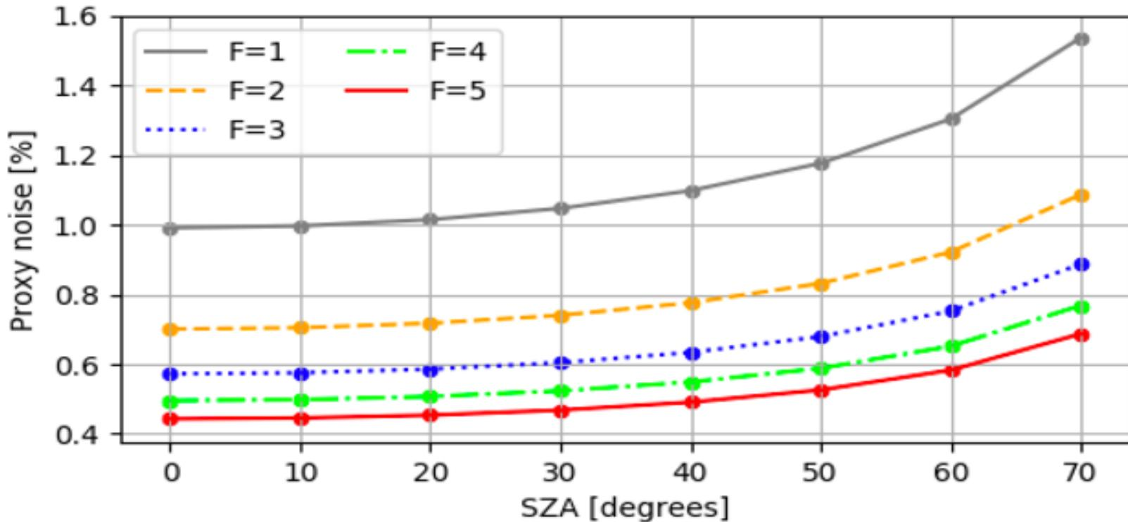
Corresponding  $\text{CO}_2$  and  $\text{CH}_4$  proxy noise for HgCdTe (MCT) detector and different forward motion compensation (F).
