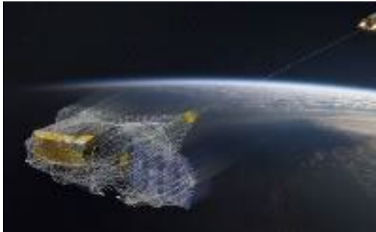
ESA's e.Deorbit mission is developing robotic arms and nets to capture Envisat (©ESA)
