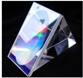
Carbonsat EE-7 grating (backup for CO2M ) (courtesy IOF-DE)
