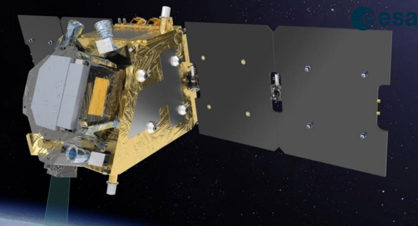
ESA's 8<sup>th</sup> Earth Explorer (FLuorescense EXplorer – FLEX) will be deployed in 2025 Will carry a high-resolution imaging spectrometer Designed to provide global maps of vegetation fluorescence that can reflect photosynthetic activity and plant health and stress
