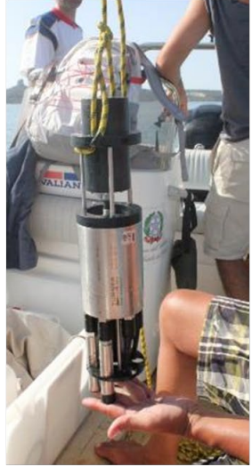
Water turbidity and fluorimetric measurements of phytoplankton pigments during fieldworks
