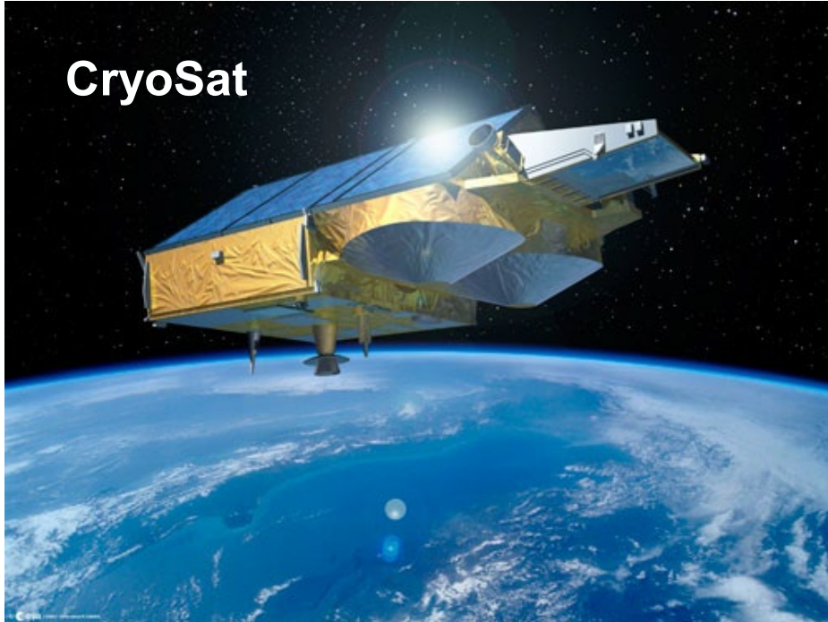
Cryosat Payload Synthetic aperture Interferometric Radar ALtimeter (SIRAL), the first of its kind
