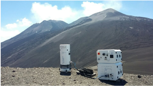
Absolute Quantum Gravimeter ( \Delta g/g \approx 10^{-9} )
