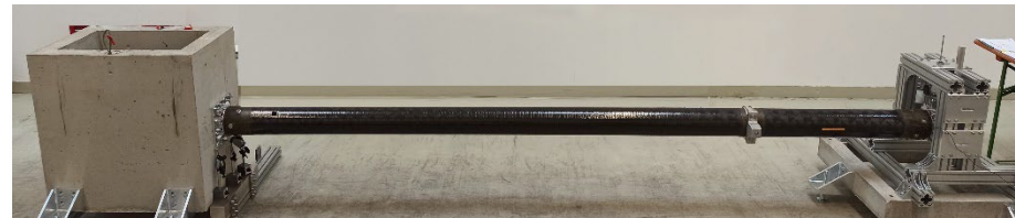
LEA-K8r Arm EM (LADEA) Mechanical Stiffness and Electrical Test at HPS, Germany
