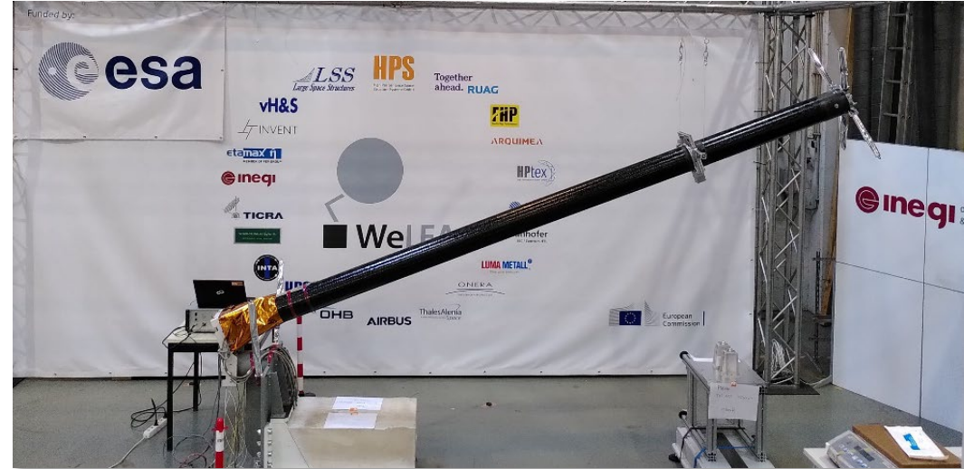
LEA-K8r Arm EM (LADEA) Deployment Test at INEGI, Portugal (April 2021)
