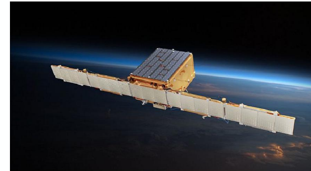
Iceye X-band SAR (85 kg satellite)
