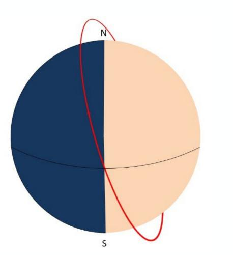
The selected orbit for the satellite is a sun synchronous polar orbit with a local time descending node at 06:00 (dawn-dusk orbit) and an orbital height of 450 km.
