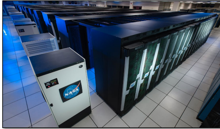
Pleiades: 9.2 PF; 11,141 CPU-nodes; 121 GPU-nodes
