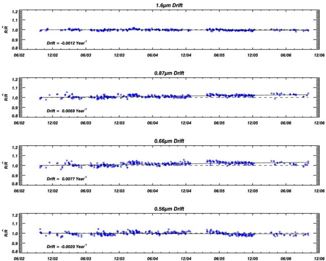
**Figure 8:** Time series of the normalised AATSR reflectances over the Sudan1 site corrected using a thin film interference drift model.
