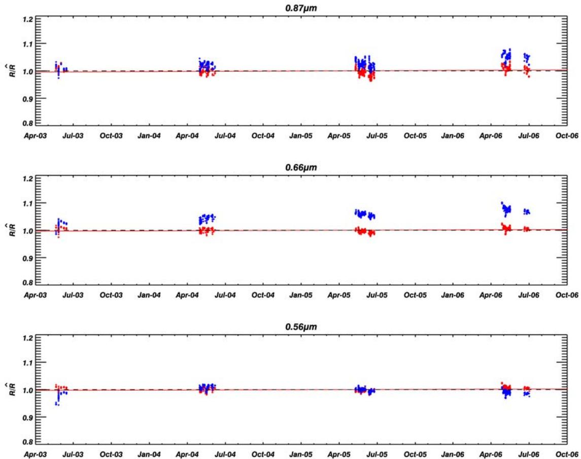
**Figure 9:** AATSR normalised radiances corrected for long term drift using the thin film model, compared against coincident measurements obtained from MERIS data, for the Greenland site.
