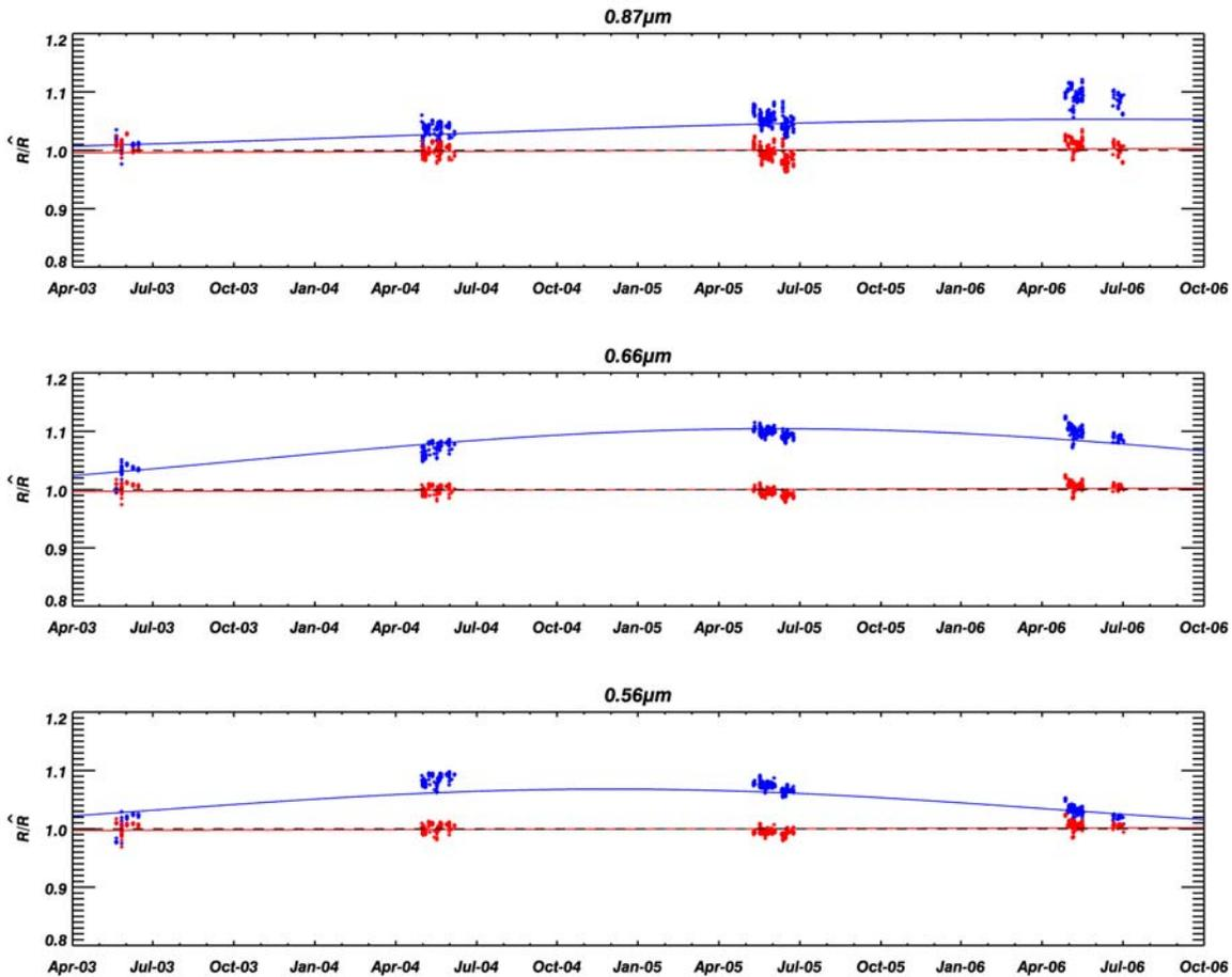
**Figure 7:** Comparison of AATSR and MERIS drifts using data from the Greenland ice-cap after removing the exponential long term drift correction. A thin film interference model has been fitted to the AATSR measurements.
