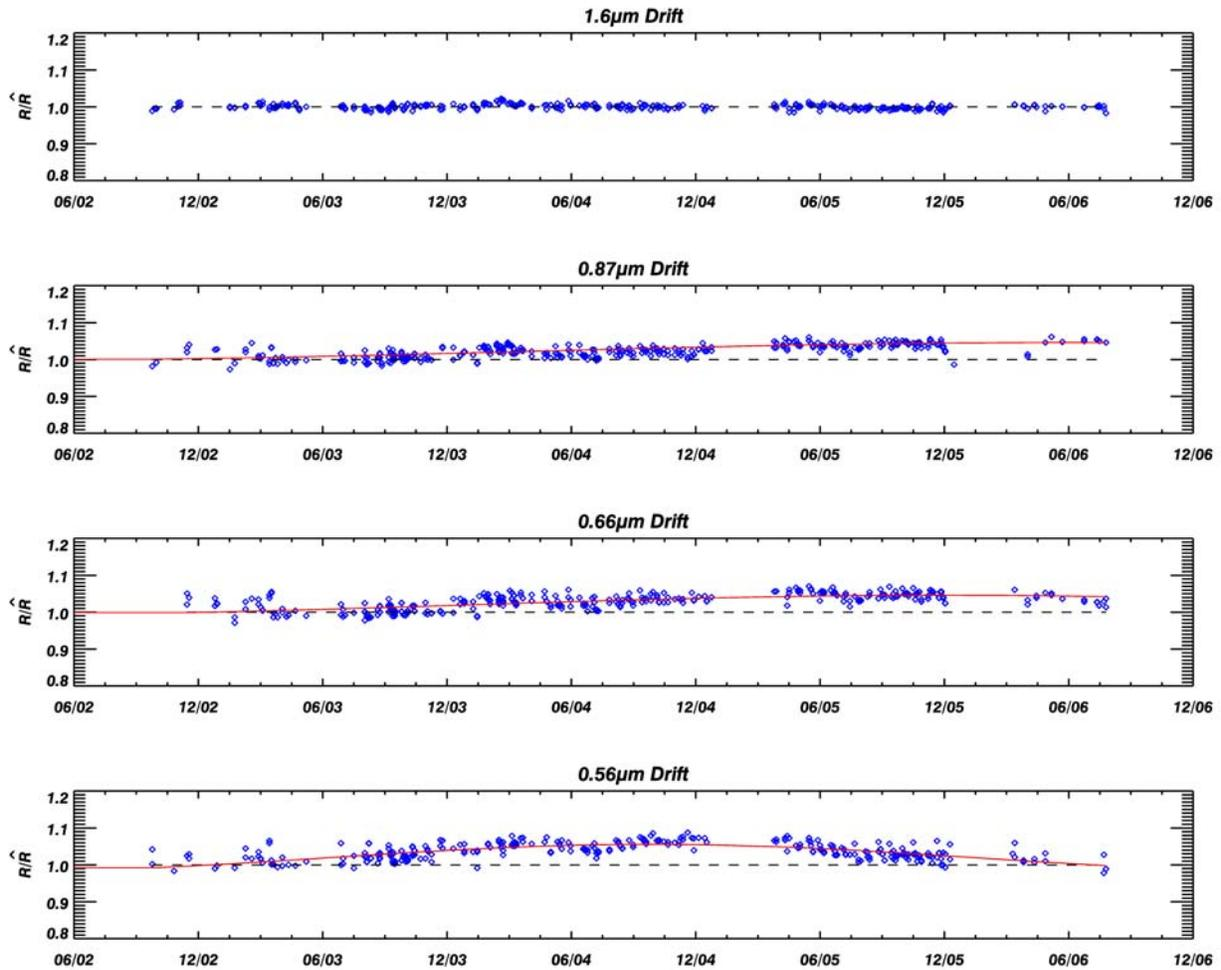
**Figure 6:** Results of fitting thin film interference model to normalised radiances for SUDAN1 test site. Note that the previous long term drift correction has been first removed from the L1B radiances (i.e. data are uncorrected before fitting)
