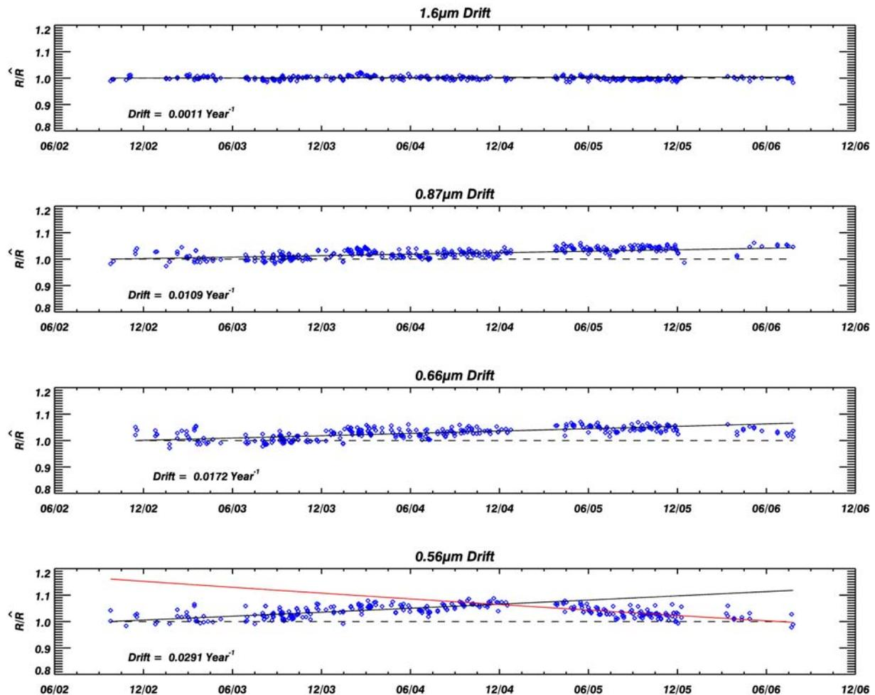
**Figure 4:** Time series of the AATSR reflectances  $R$ , normalised to a Bidirectional Reflectance Distribution Function,  $\hat{R}$  for the Sudan1 site over the time period up to 2006, showing the change in direction of the  $0.56\mu\text{m}$  drift.
