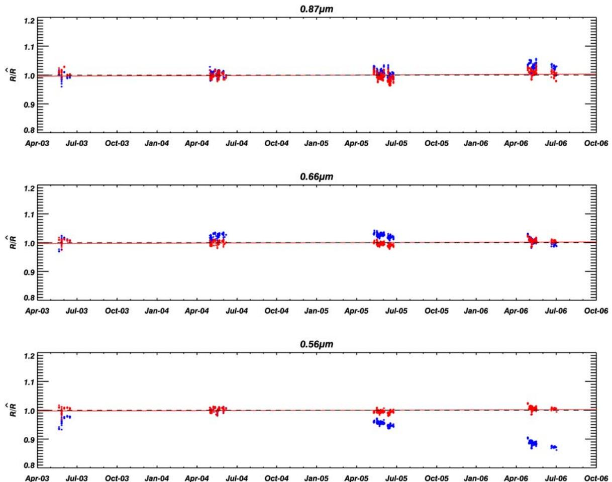
**Figure 3:** Comparison of AATSR and MERIS drifts using data from the Greenland ice-cap. Here the BRDF, has been obtained by least squares fit of MERIS reflectance vs. cosine solar zenith angle.
