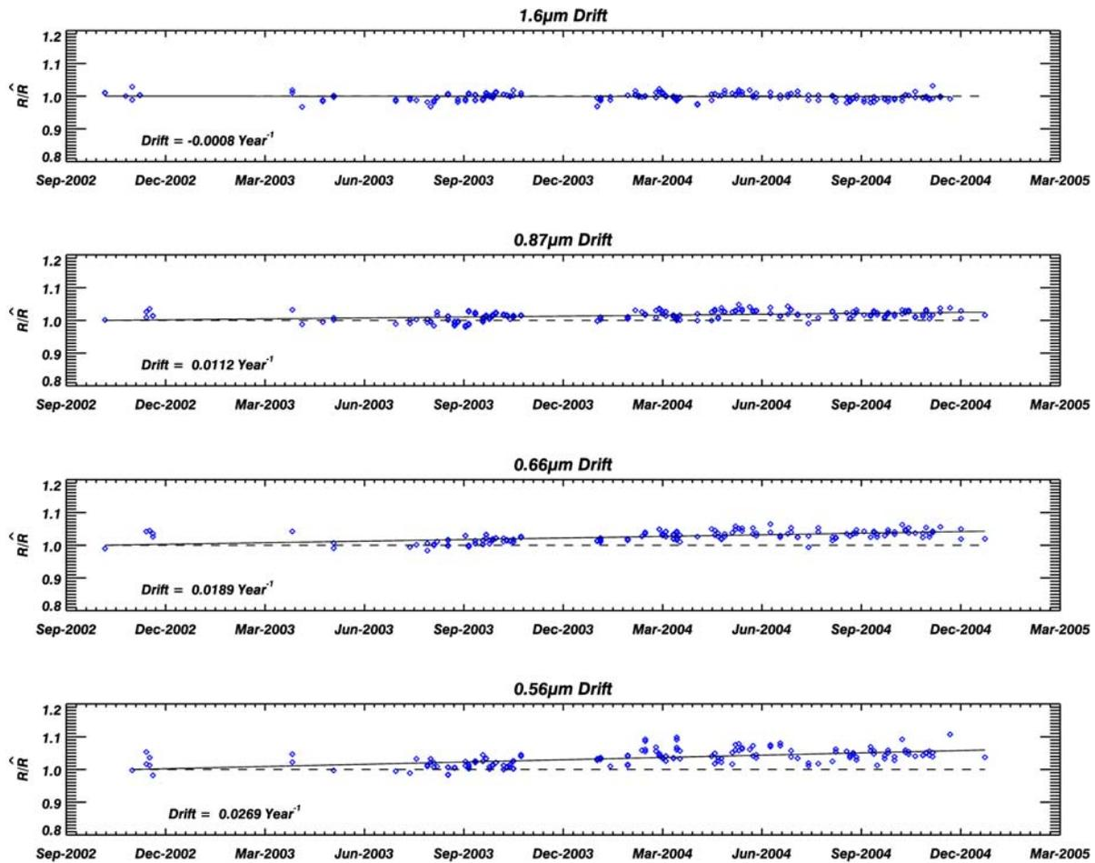
**Figure 1** - Time series of the AATSR reflectances  $R$ , normalised to a Bidirectional Reflectance Distribution Function,  $\hat{R}$  over the Arabia1 site. Here the BRDF is obtained by fitting to the AATSR TOA reflectances as a function of scattering angle.
