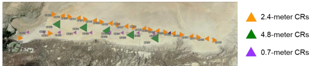
Figure 3-1: Corner reflectors in Rosamond calibration site, California
