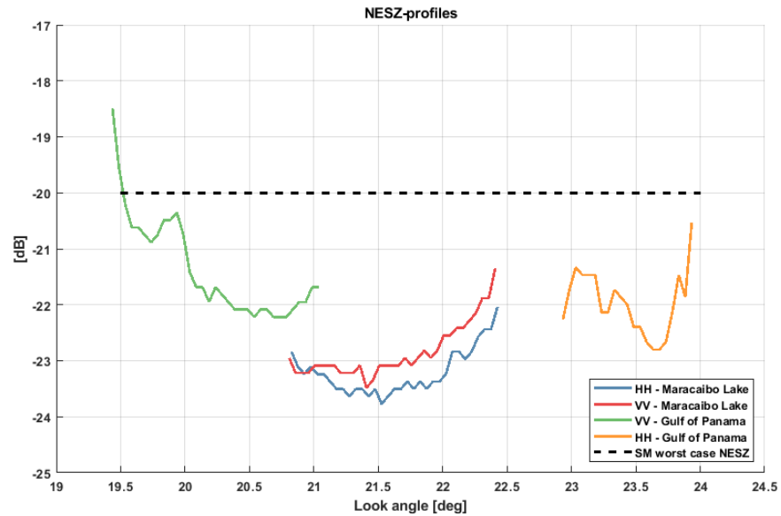
Figure 4-13: Results of sensitivity analysis: NESZ profiles measured from acquisitions over calm water areas compared to the NESZ level as measured during the payload calibration performed in June 2022 and reported in [RD-6].
