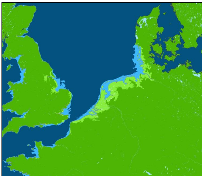
Figure 42: Example of mask alignment. Ocean areas from land/ocean mask in dark blue; Coastline mask in red; Tidal regions mask intersecting with water mid blue; Water from land/water mask light blue and land dark green; Land intersecting with tidal region mask light green.
