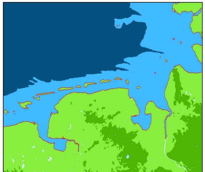
Figure 42: Example of mask alignment. Ocean areas from land/ocean mask in dark blue; Coastline mask in red; Tidal regions mask intersecting with water mid blue; Water from land/water mask light blue and land dark green; Land intersecting with tidal region mask light green.
