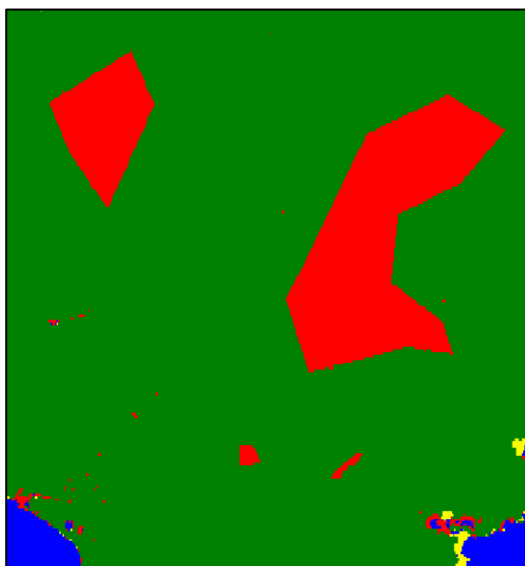
Figure 20: Differences between CCI water body mask and BEAM SRTM water fraction (left) [green = land in both masks; blue = water in both masks; red = water in CCI WB and land in BEAM SRTM/S3; yellow = water in BEAM SRTM/S3 and land in CCI WB]; Satellite image (right – source: Google Earth).
