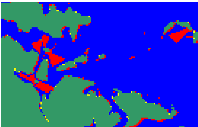
Figure 11: Differences between CCI water body mask and BEAM SRTM water fraction (left) [green = land in both masks; blue = water in both masks; red = water in CCI WB and land in BEAM SRTM/S3; yellow = water in BEAM SRTM/S3 and land in CCI WB]; Satellite image (right – source: Google Earth).
