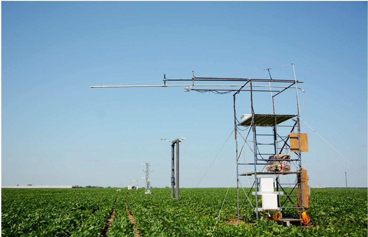
Figure 4: Mounting of D-FloX and other SIF sensors.
