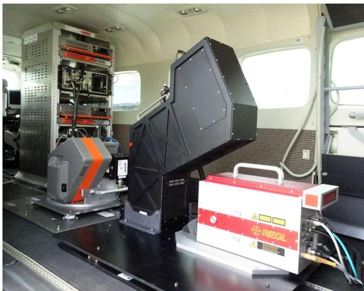
Figure 7: TASI-600 and laser scanner (LiDAR) Riegl LMS-Q780 mounted in the aircraft together with HyPlant.
