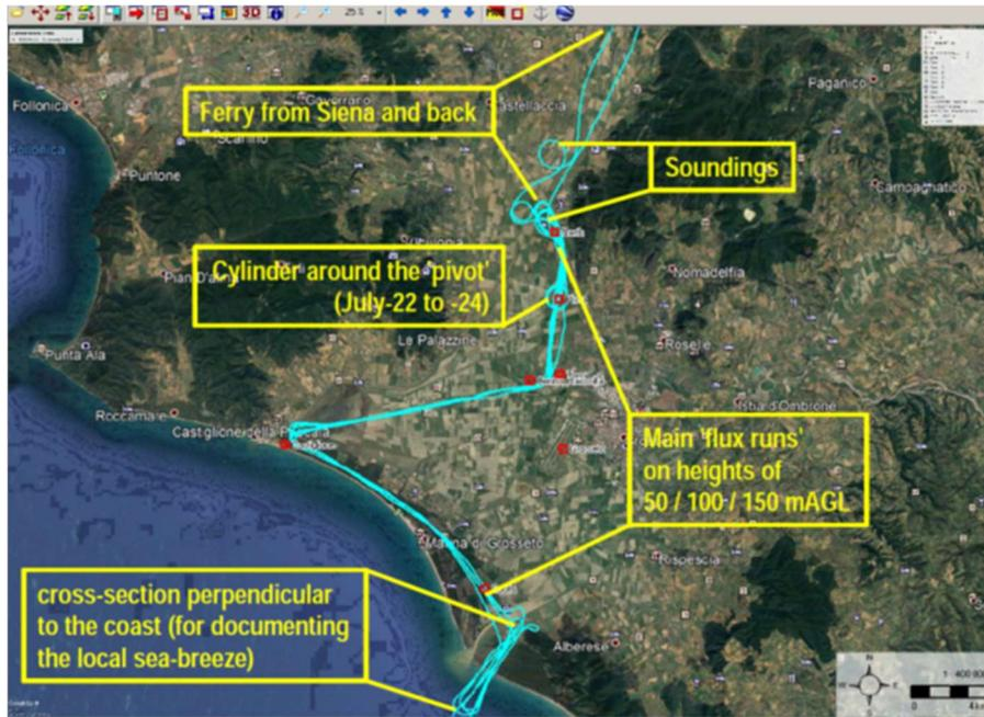
Figure 8: Standard flight pattern for Grosseto, Italy. This pattern was repeated up to five times (back and forth) per day (about half an hour per completed run).
