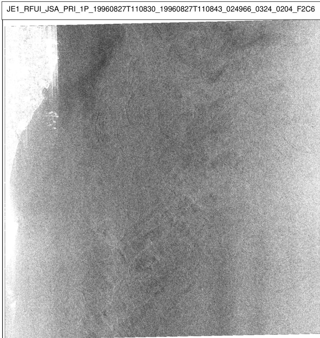
**Figure 4-1: PRI product with faint azimuth ambiguities on the left side of the image, an artefact of the bright land.**
