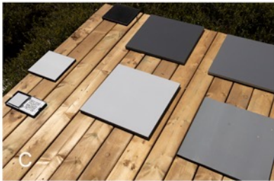
Figure 2. (A) Altum mounted on the M300. (B) Mjolnir VS-620 hyperspectral sensor mounted on an octocopter with a gimbal for stabilization. (C) Six diffuse reflectance panels (2%, 5%, 10%, 18%, 40%, 50%) and the included MicaSense calibration reflectance panel. (D) HR1024i spectroradiometer taking field measurements of diffuse reflectance panels.
