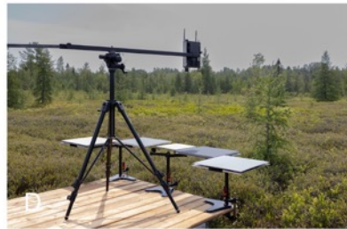
Figure 2. (A) Altum mounted on the M300. (B) Mjolnir VS-620 hyperspectral sensor mounted on an octocopter with a gimbal for stabilization. (C) Six diffuse reflectance panels (2%, 5%, 10%, 18%, 40%, 50%) and the included MicaSense calibration reflectance panel. (D) HR1024i spectroradiometer taking field measurements of diffuse reflectance panels.
