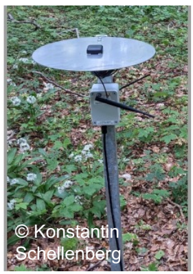
Antenna: RS ANT-GPSC Receiver: ublox NEO-M9N
