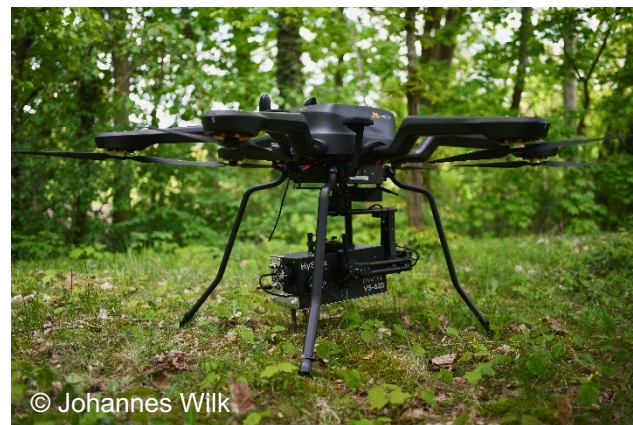
GFZ Acecore Noa 6 integrated with HySpex VS-620
