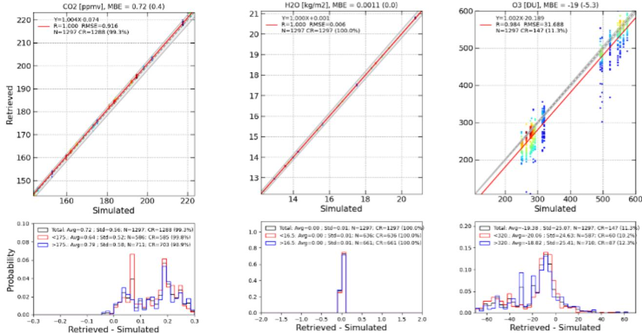
BTS direct irradiance measurements show proper sensitivity to all gaseous species but: NO<sub>2</sub> and O<sub>3</sub>
