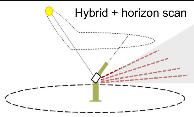
**TASK:** to simulate **near-horizon** radiometer sky scanning **observations** (e.g. **AERONET**) and test with GRASP for aerosol profiling
