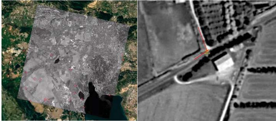
Figure 2-1: (Left) The number and distribution of coverage of ground control points (+) from the field survey conducted in the area of La Crau, France. (Right) As an example, the apparent location of a ground control point (x) is located in the product image (e.g. panchromatic band) and the displacement is calculated by determining the difference between the true and apparent location.
