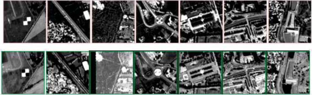
Figure 2-8: Image clips of a small collection of points of interest from the panchromatic band of a target sensor and reference sensor .
