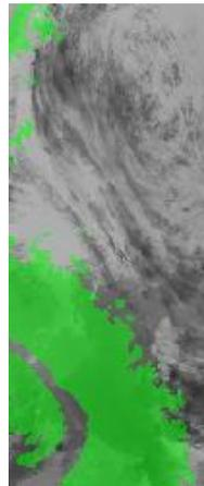
**Figure 2-4. An example of the land flag (green) set in the 12  $\mu\text{m}$  nadir BT channel.**
