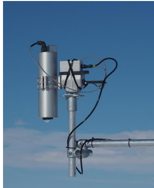
HYPSTAR® system [https://hypstar.eu] 380-1700nm, 3-10nm FWHM
