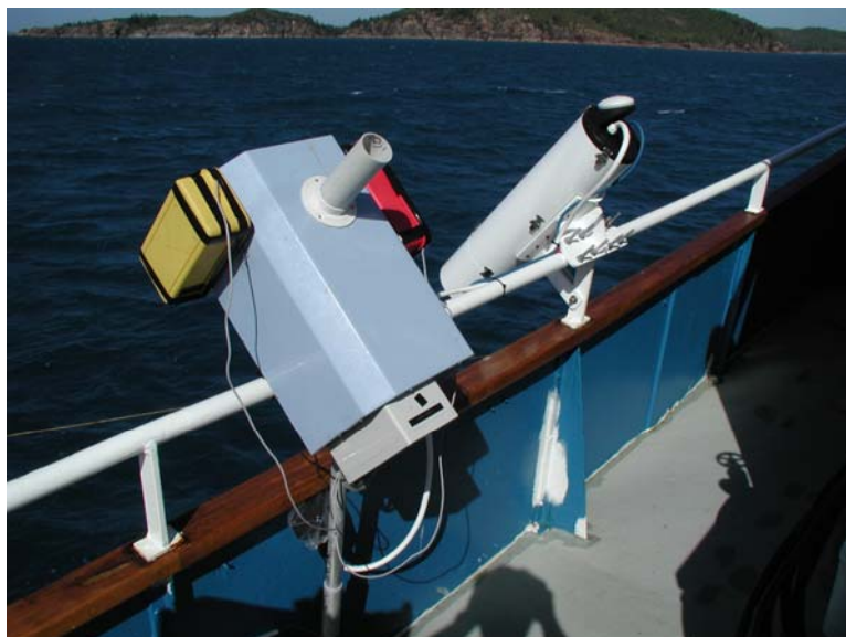
Figure 9.2.3.1-1 The DAR011 (left) and the AIMS radiometer (right) mounted on the RV Lady Basten
