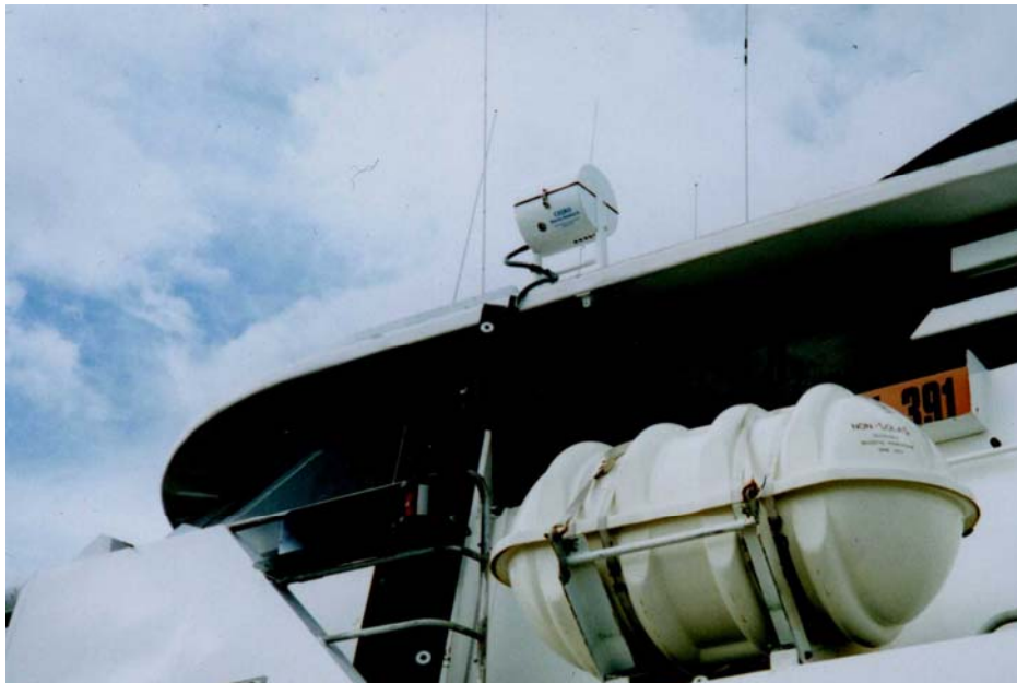
Figure 9.2.1.1-1 The new Perth radiometer mounted on the ferry "Sea Flyte"
