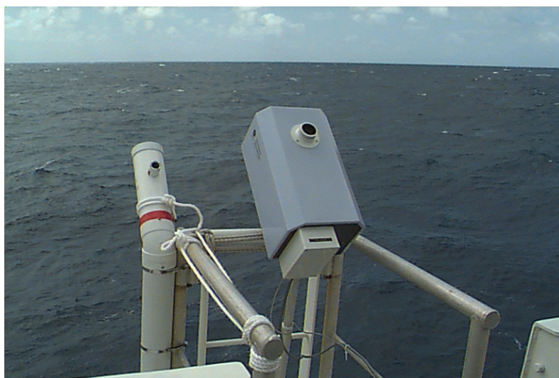
Figure 9.3.3.1-1: The DAR011 radiometer, mounted on the RV Franklin, used for validation activities based in Hobart (Photograph from CSIRO)
