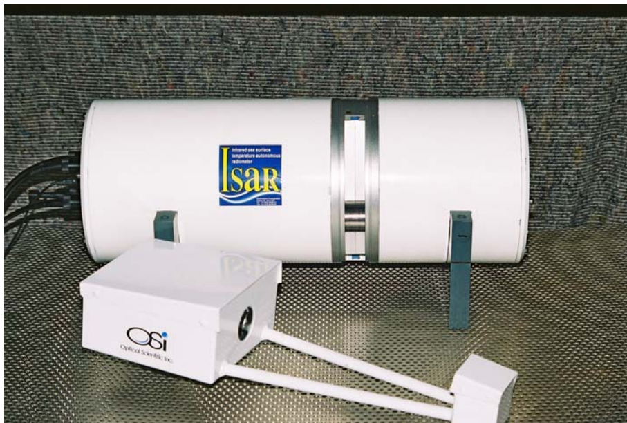
Figure 9.2.1.1-1 The Infrared Autonomous SST Radiometer (ISAR5C) shown together with the optical rain gauge. The rain gauge is used to control the opening/closing of a shutter system that seals the instrument from rain and sea spray during bad weather.
