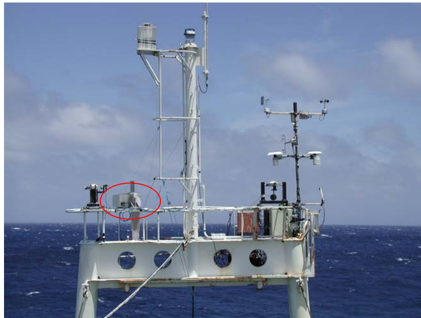
Figure 9.3.1.1-1 SISTeR mounted on the foremast platform of the RSS Charles Darwin
