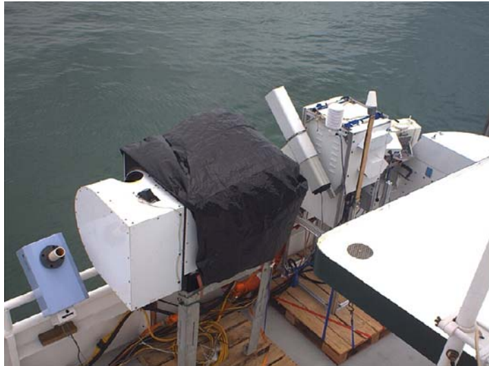
Figure 9.3.2.2-1 View from above of the radiometers mounted on the R/V Walton-Smith. From fore to aft, they are the SISTeR, ISAR5C (hidden), CIRMS, M-AERI and DAR011
