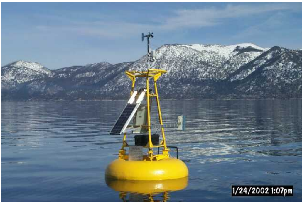
Figure 11.1.5.1-2. Surface monitoring station at TR1. The station measures the radiometric skin temperature, bulk temperature, wind direction (magnetic) and speed, relative humidity, air temperature and net radiation.
