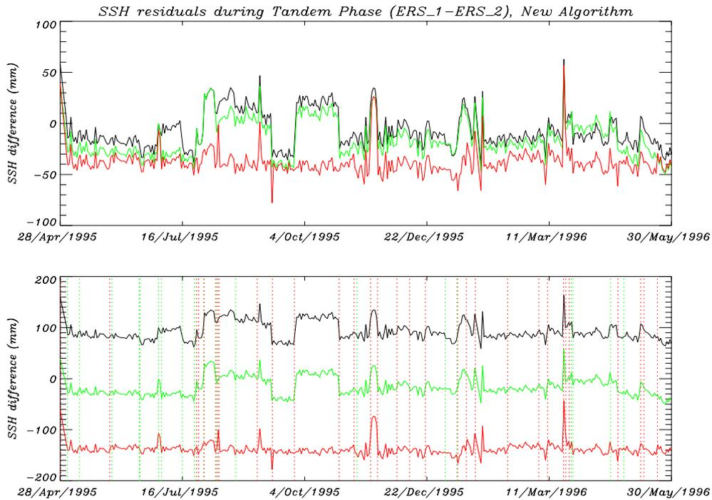
**Figure 3:** SSH difference (ERS\_1-ERS\_2) during Tandem Phase. Validation results for new range correction algorithm.
