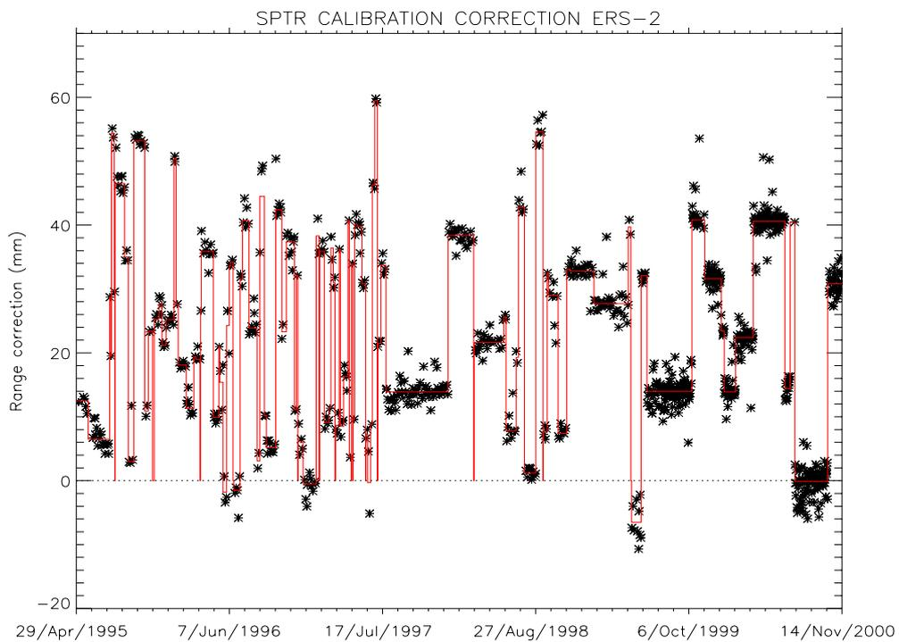
**Figure 2:** SPTR measurement values and final range correction for the whole ERS-2 mission
