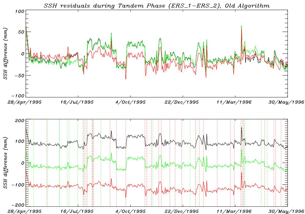
**Figure 4:** SSH difference (ERS\_1-ERS\_2) during Tandem Phase. Validation results for new range correction algorithm.
