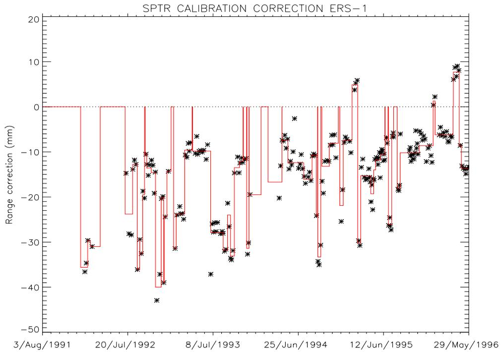
**Figure 1:** SPTR measurement values and final range correction for the whole ERS-1 mission
