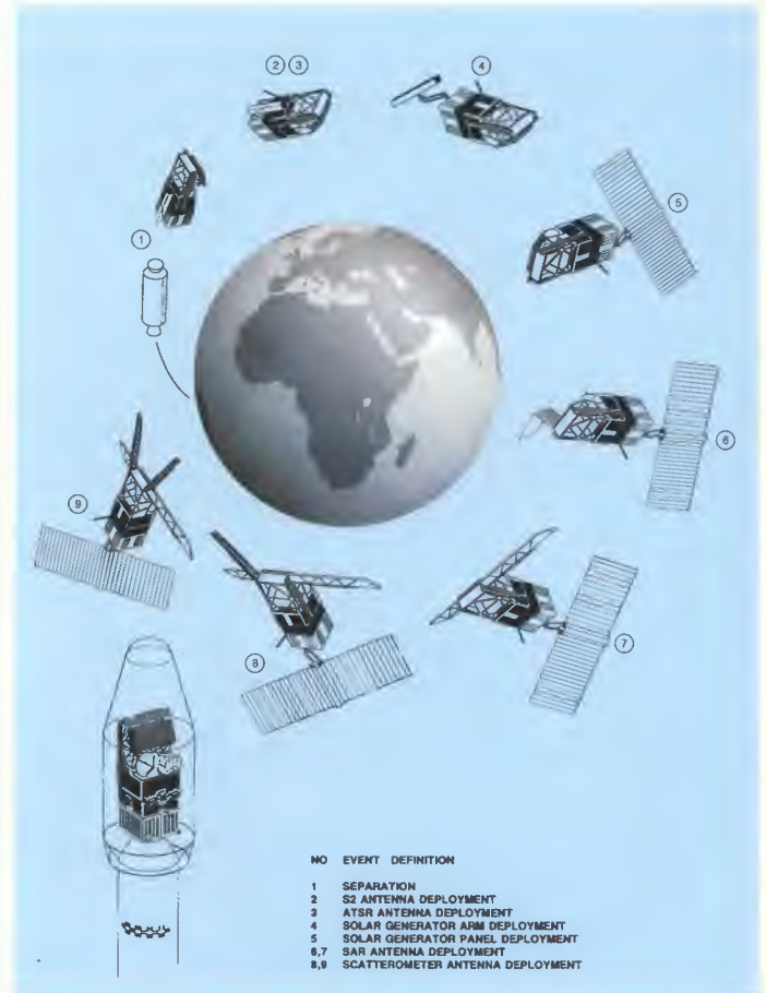
Nominal operational sequence for the Launch and Early Orbit Phase (LEOP)
