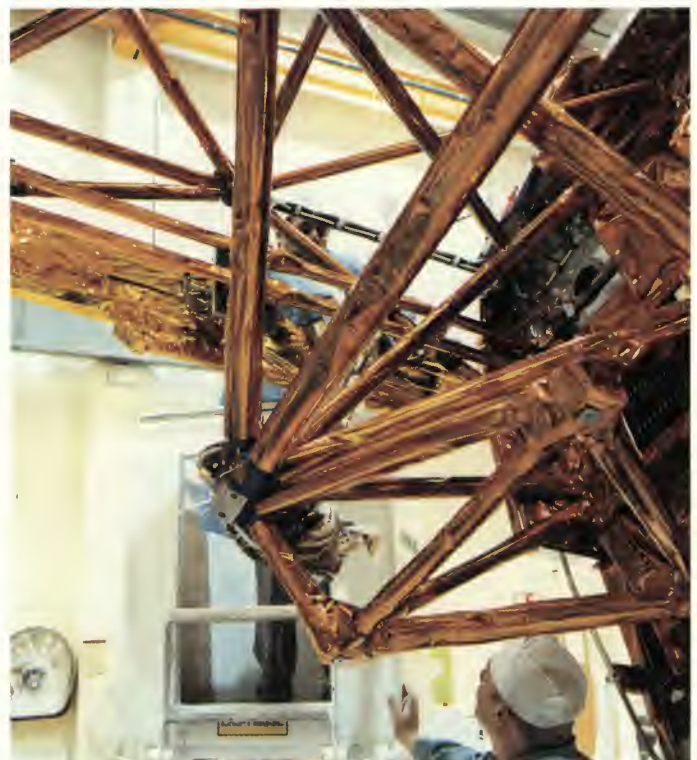
Part of the Antenna Support Structure (ASS) with the antennas removed
