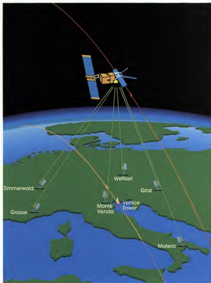
Calibration of the Radar Altimeter by comparing measured height over the Northern Adriatic with laser-ranging measurements from an array of laser stations
