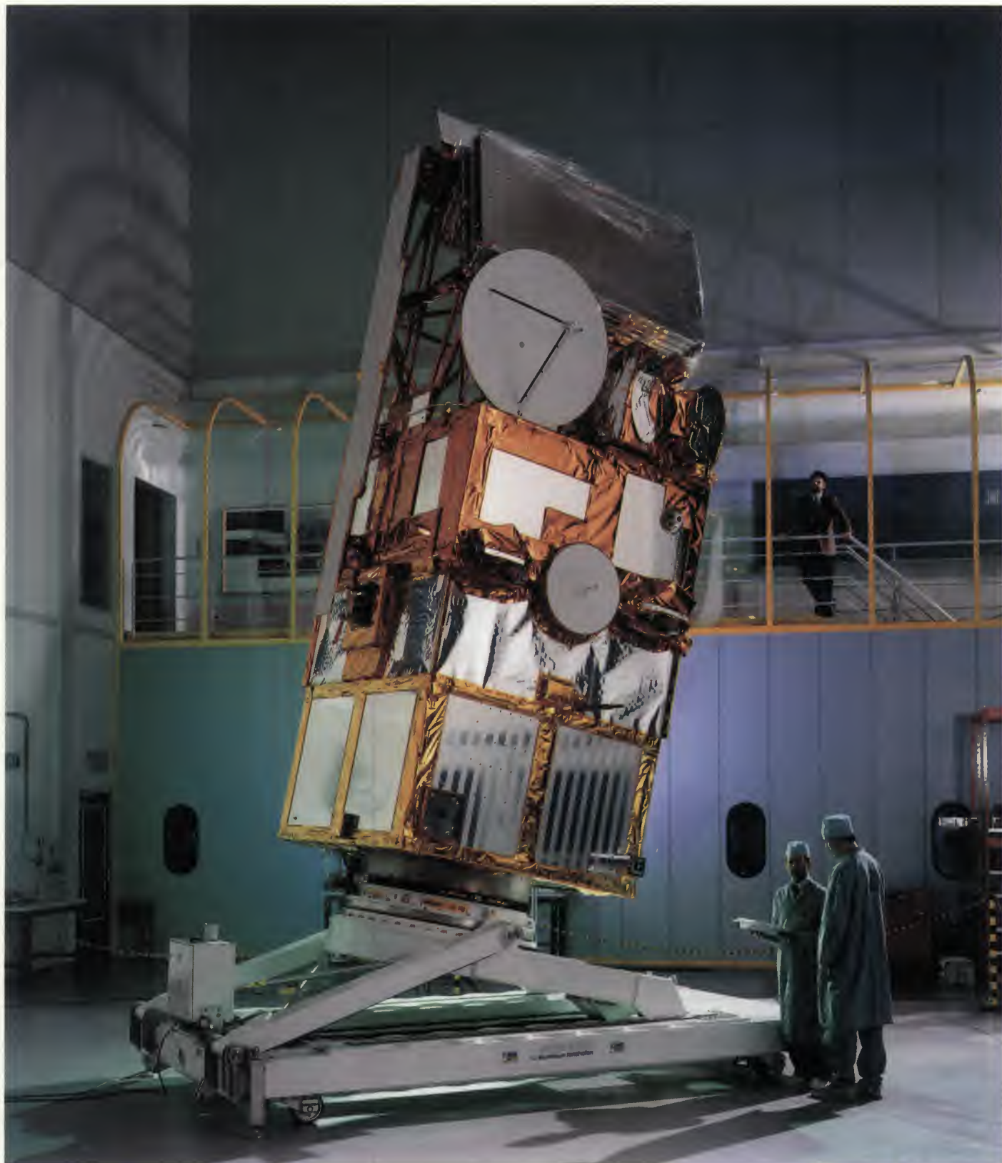
The ERS-1 spacecraft in launch configuration, the arrays and antennas folded, during tests at the European Space Agency's ESTEC facilities, in Noordwijk, The Netherlands
