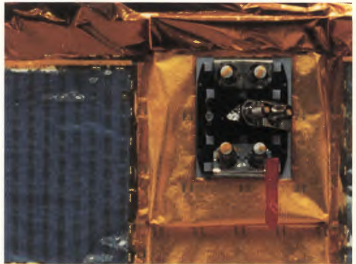
The thrusters on the flight model of ERS-1
