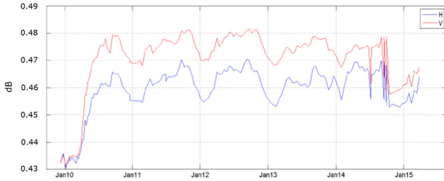
Fig. 16. Evolution of the antenna losses as measured in flight.
