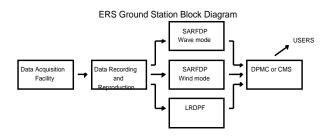
Figure 2: ERS Ground Station Block diagram
