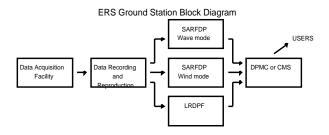
Figure 3: ERS Ground Station Block diagram
