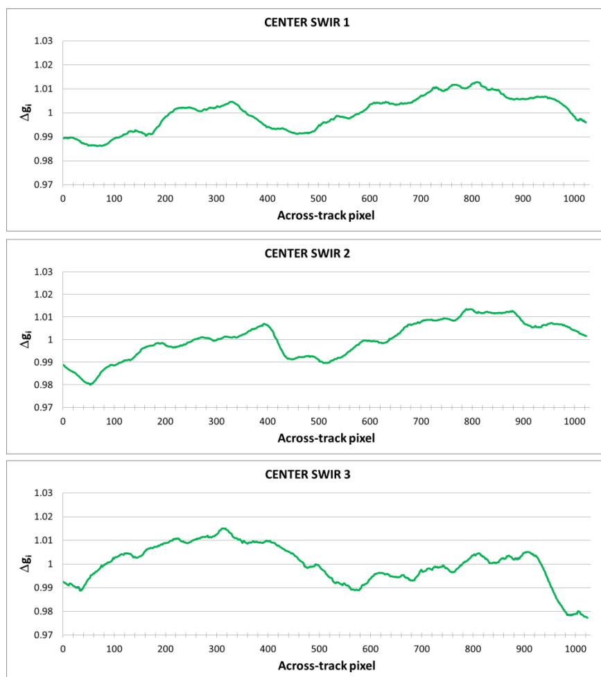
Figure 41: Changes to the equalisation over the field of view. A value lower than 1 results in an increase in the TOA reflectance while a value higher than 1 gives a TOA reflectance decrease.
