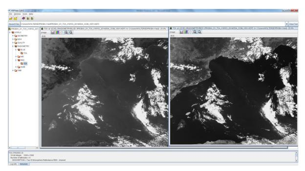
Figure 20: Overview of the Datasets, Groups, and images of the BLUE and RED spectral bands within a PROBA-V L1C HDF5 file.
