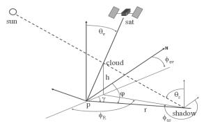
Figure 10: Depiction of solar, satellite, cloud, and cloud shadow geometries.
