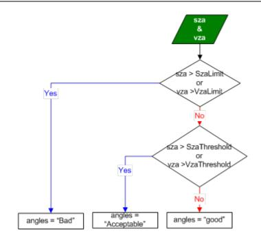
Figure 13: Procedure to determine the observation quality based on SZA and VZA in the synthesis processing. Note that in the 1 km processing only the SZA rule is applied.
