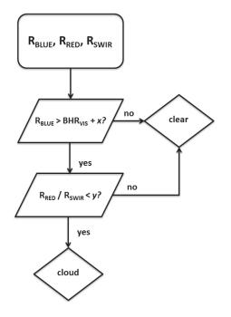
Figure 9: Flowchart of the proposed cloud detection algorithm modification. Variables 'x' and 'y' refer to the reflectance added to the spatially corresponding surface albedo value and RED over SWIR threshold values, respectively.
