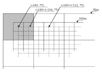
Figure 28: 1km and 300m plate-carrée grids
