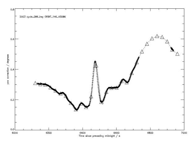
Figure 4: Interpolation and extrapolation of HEY data. Symbols: ++ HEY data,  $\Delta\Delta$  HEY "stack" (spline fit, 30s samples), -- HEY data (reconstructed from stack). Each end of the curve is extended (to the next sample point) by "external" extrapolation using a linear fit to the last 10 data points. The large gap towards the right-hand side is filled by interpolation using the spline fit.
