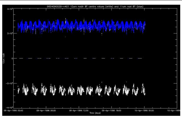
Figure 23: Centre of scan brightness temperatures for the whole day of 09-Apr-1996, 12µm and 11µm channels, from the updated SUPPLE processor.
