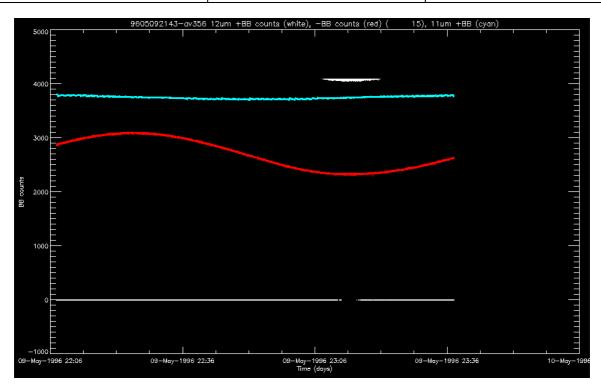
Figure 14: Counts from the 12µm channel warm (white) and cold (red) blackbodies and from the 11µm channel warm blackbody, for the orbit at 21:43 09-May-1996
