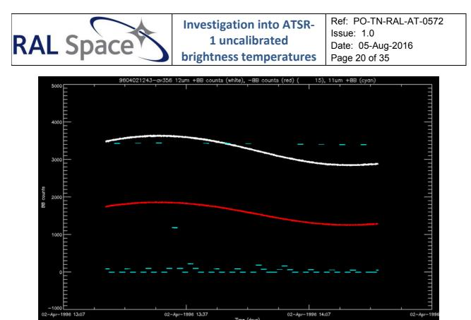
Figure 13: Counts from the 12µm channel warm (white) and cold (red) blackbodies and from the 11µm channel warm blackbody, for the orbit at 02-Apr-1996 12:43.
