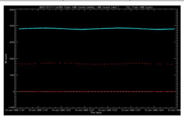
Figure 10: Counts from the 12µm channel warm (white) and cold (red) blackbodies and from the 11µm channel warm blackbody, for the orbit at 1996-01-10 11:11
