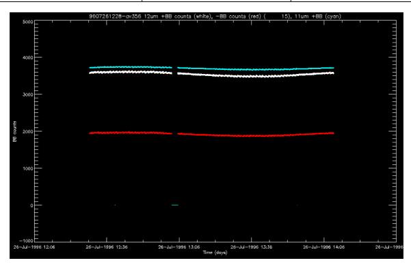
Figure 19: Counts from the 12µm channel warm (white) and cold (red) blackbodies and from the 11µm channel warm blackbody, for the orbit at 12:28 26-Jul-1996.
