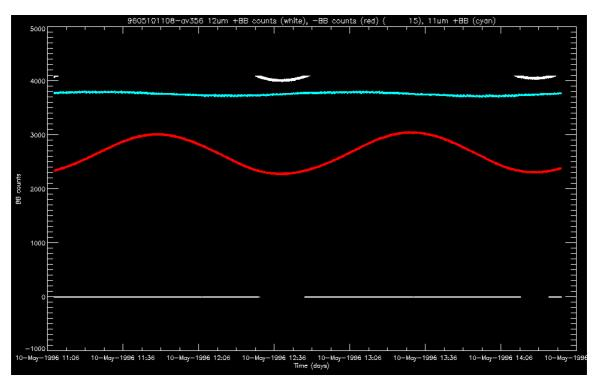
Figure 16: Counts from the 12µm channel warm (white) and cold (red) blackbodies and from the 11µm channel warm blackbody, for the 2 orbits at 11:08 10-May-1996
