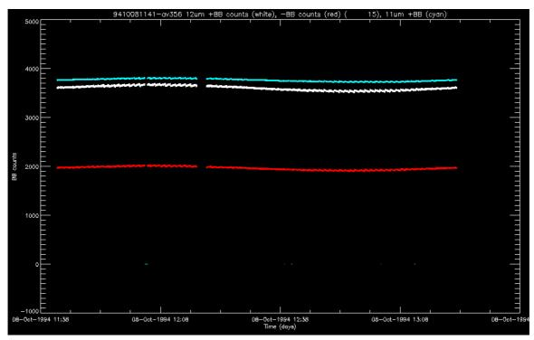
Figure 9: Counts from the 12µm channel warm (white) and cold (red) blackbodies and from the 11µm channel warm blackbody, for the orbit at 11:41 08-Oct-1994
