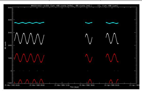
Figure 11: Counts from the 12µm channel warm (white) and cold (red) blackbodies and from the 11µm channel warm blackbody, for several orbits on 1996-03-31
