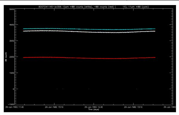
Figure 5: Blackbody counts from the 12µm channel warm (white) and cold (red) blackbodies and from the 11µm channel warm blackbody, for the orbit from 24-Jul-1992 11:45.
