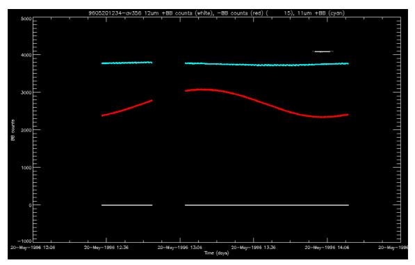
Figure 17: Counts from the 12µm channel warm (white) and cold (red) blackbodies and from the 11µm channel warm blackbody, for the orbit at 12:34 20-May-1996
