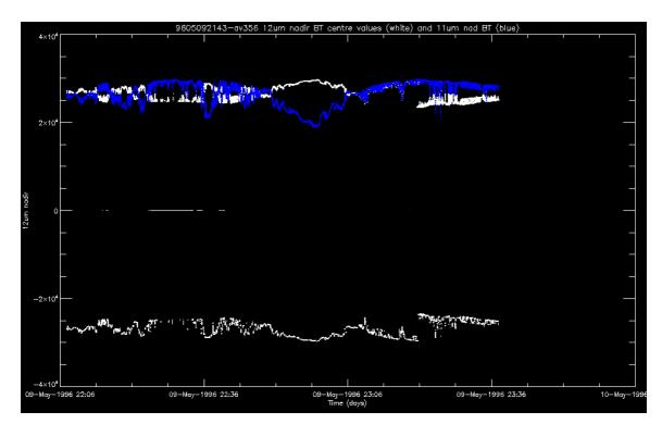
Figure 15: Brightness temperature values from (approximately) the centre of scan for orbit at 21:43 09-May-1996. 12µm values in white, 11µm blue
