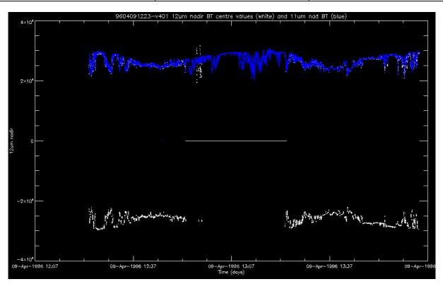
Figure 21: Centre of scan brightness temperatures for the 12µm and 11µm channels, from the updated SUPPLE processor.
