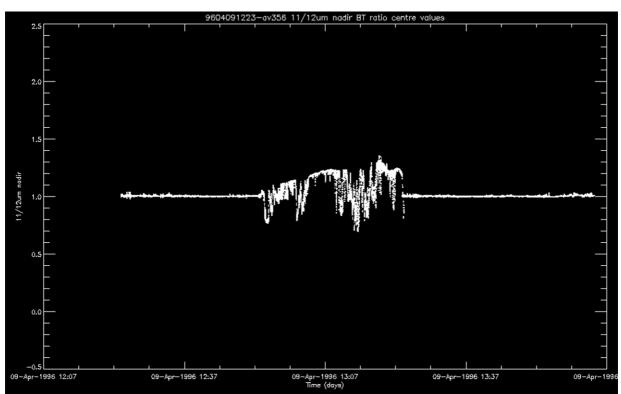
Figure 3: Ratio of the centre-scan brightness temperatures in the 11µm and 12µm channels, for the orbit from 09-Apr-1996 12:23.
