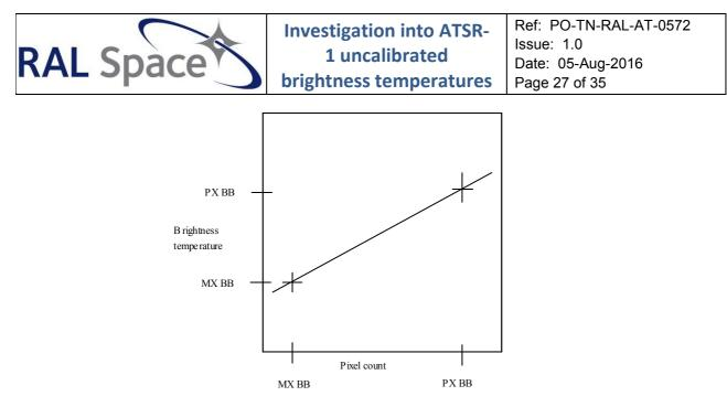
Diagramatic representation of the linear calibration of pixel counts to brightness temperature
