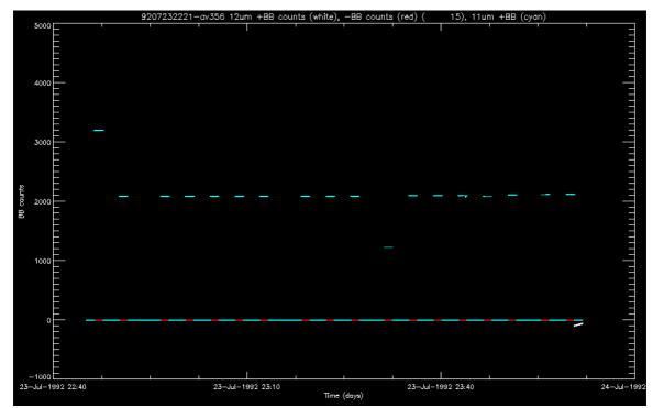
Figure 4: Blackbody counts from the 12µm channel warm (white) and cold (red) blackbodies and from the 11µm channel warm blackbody, for the orbit from 23-Jul-1992 22:21
