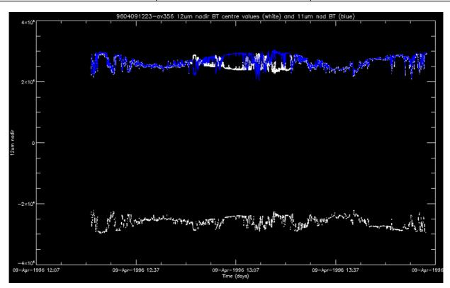
Figure 2: Brightness temperature values from (approximately) the centre of scan for orbit at 12:23 09-Apr-1996. 12 $\mu$ m values in white, 11 $\mu$ m in blue. The lower white trace with negative values is caused by blanking pulse flags in the data.
