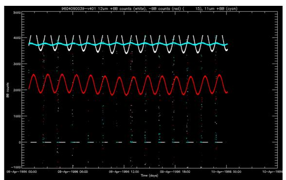
Figure 12: Blackbody values from the full day's data for 09-Apr-1996, showing the extent of blackbody saturation. (Same colours as Figure 1, 12µm warm blackbody counts are shown in white)
