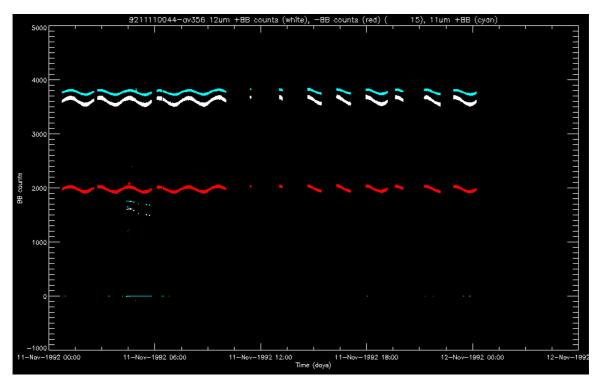
Figure 6: Counts from the 12µm channel warm (white) and cold (red) blackbodies and from the 11µm channel warm blackbody, for all available UBT files on 11-Nov-1992
