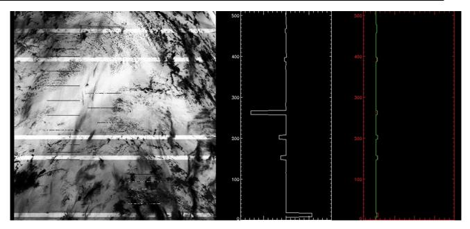
Figure 11: UBT channel image containing band artefacts, with line plots of the odd/even gain ratio in each row and the individual odd/even gain values
