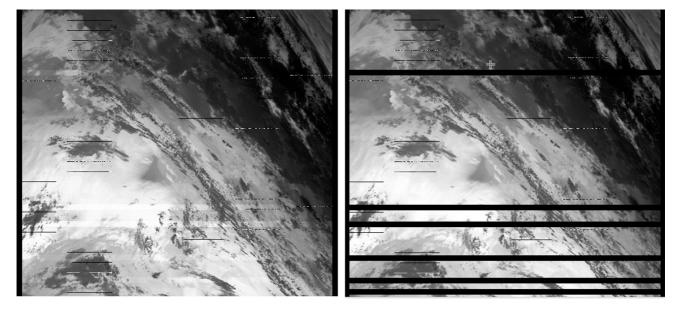
Figure 12: a UBT image affected by band features (left) and the result of an experimental pixel flagging based on the odd-even gain ratio (right)
