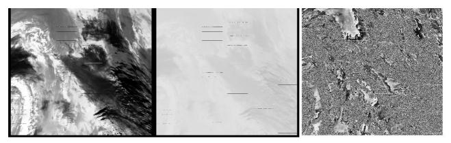
Figure 2: 3 image display options for the 11µm nadir channel. Left to right: histogram-equalised, tvscl (raw image), tv (raw image).
