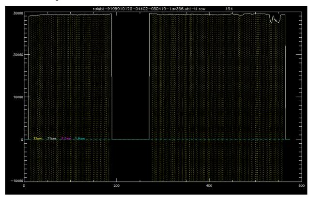
Figure 4: plot along a scan containing a "dash" artefact, showing all channels. The dotted lines alternating from positive to negative values are caused by the negation of 12µm channel values to indicate the presence of the blanking pulse.
