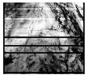
Figure 13: a UBT scene in which the attempted flagging based on odd-even gain ratio did not remove all band features.
