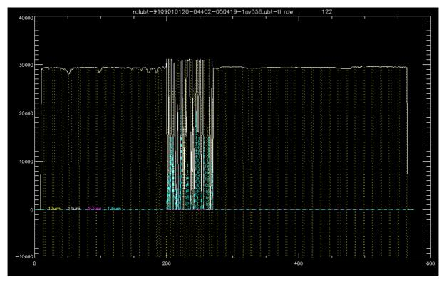
Figure 7: pixel values in a scan line containing a "dotted dash" artefact
