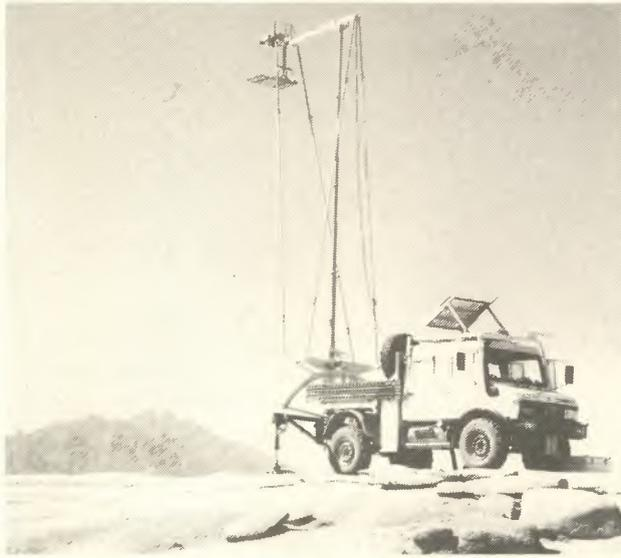
Figure 6: Ground truth vehicle with extended hydraulic mast during field work.
