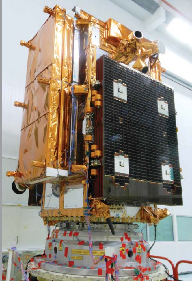
Sentinel-1A on the vibration shaker at the Thales Alenia Space test facilities, Cannes (Thales Alenia Space)
