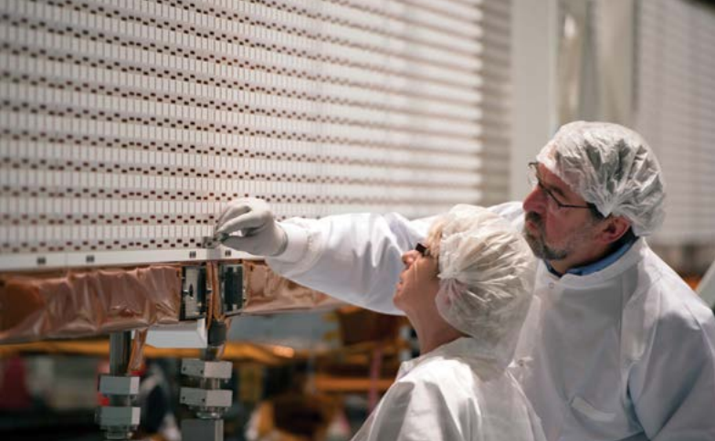
Testing the deployment of the Sentinel-1A radar antenna in the cleanroom at Thales Alenia Space in Cannes, France
