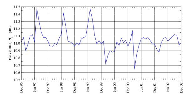
Figure 16: Monthly global mean of ERS-2 RA backscatter coefficient after QC during the period from December 1996 to December 2002.
