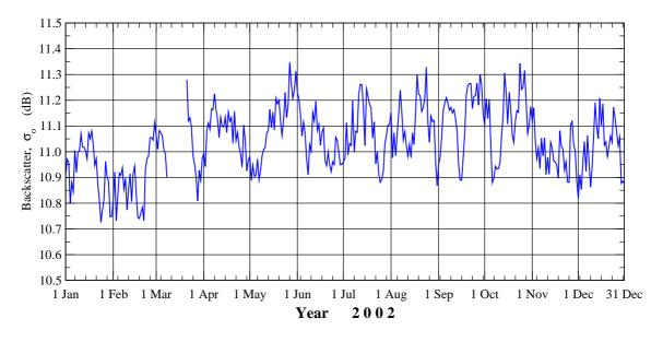
Figure 15: Daily global mean of ERS-2 RA backscatter coefficient after QC during the whole year of 2002.
