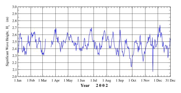
Figure 2: Daily global mean of ERS-2 RA significant wave height after QC during the whole year of 2002.
