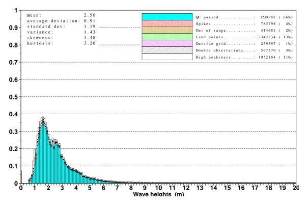
Figure 1: Distribution of ERS-2 RA significant wave heights after QC during the period from 21 March to 31 December 2002.
