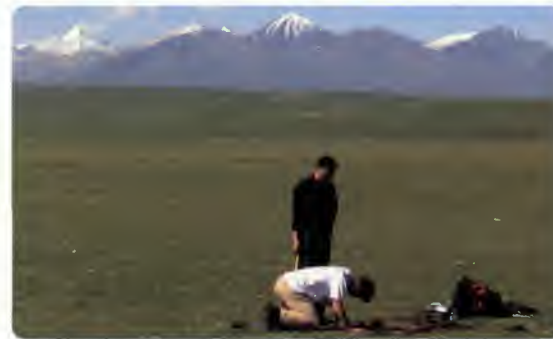
▶ Zhao Yizhou and Rogier van der Velde installing soil moisture and temperature probes at 5 different levels up to a depth of 60 cm on the Tibetan Plateau
