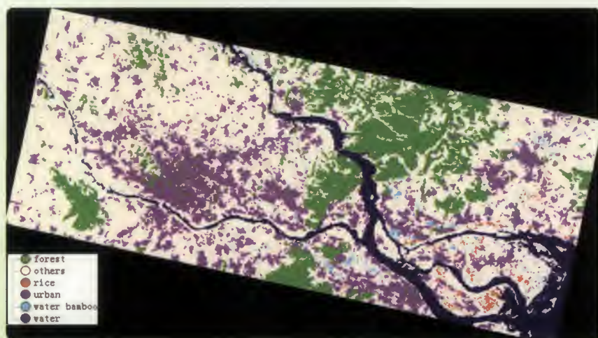
▶ Zhangzhou-classification-map: Land cover, land use classification map of Zhangzhou in 2005 by using ERS and ASAR
