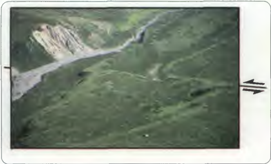
Haiyuan fault near longitude 102.75°. Left-lateral accumulated displacements shown by arrows Courtesy F. Métivier, IPGP
