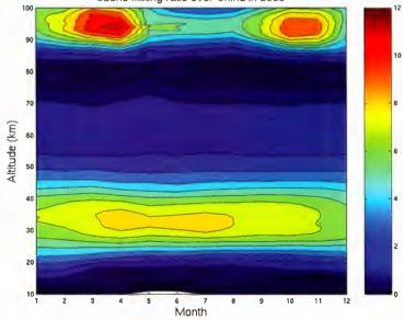
Time-evolution of the ozone profiles in the altitude region of 10-100 km in the area shown by the map above. The analysis is based on 2500 night time occultations measured by GOMOS in 2003
