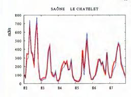
red: measured discharge blue: modelled discharge
