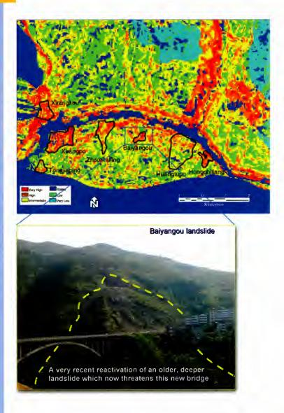
" Landslide hazard map of the Badong area, derived from geo-spatial analysis of thematic layers including slope derived from EO data. (Courtesy of Dr. Jian Guo Liu)
