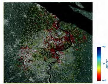
E Average displacement rate of the radar benchmarks (PS) identified from a time series of ERS SAR images in Shanghai city, P.R. China. (Courtesy of Politecnico di Milano)
