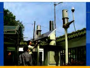
Hydrological observation stations in study catchments provide daily meteorological data that can be used to calibrate and run surface runoff models, Courtesy of Xin Jingfeng
