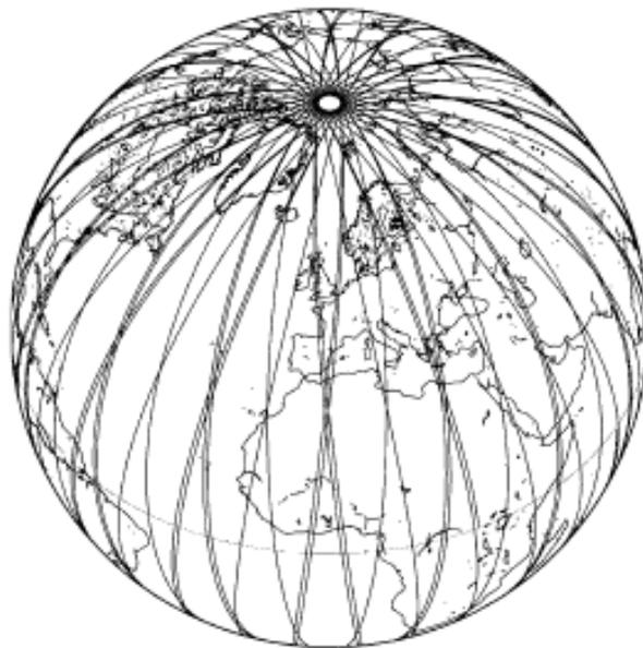
Figure 5: Example of tracks of CryoSat-2's orbit over a three-day period
