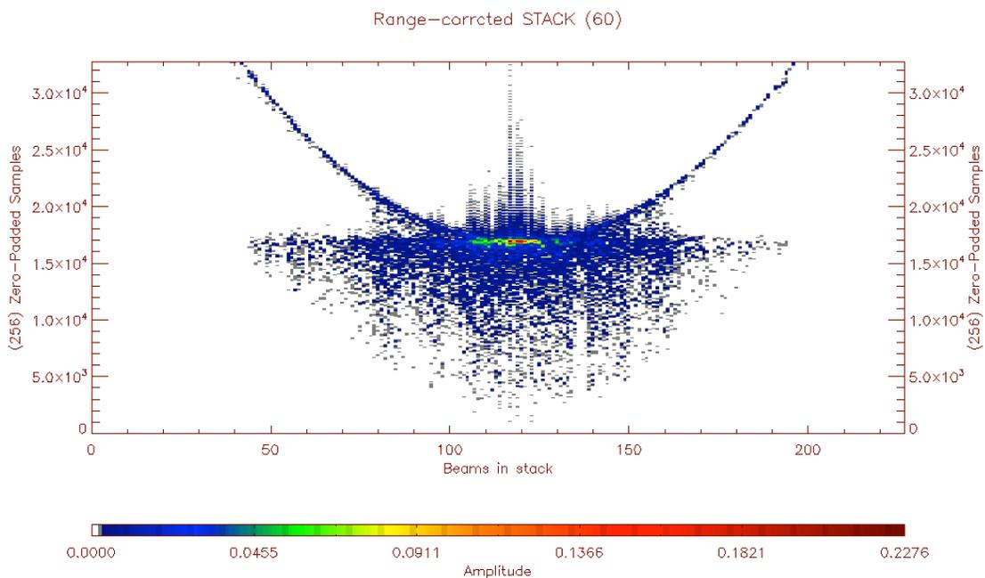
Figure 14: Stack 60 without hamming: here the parabola is the nadir clutter
