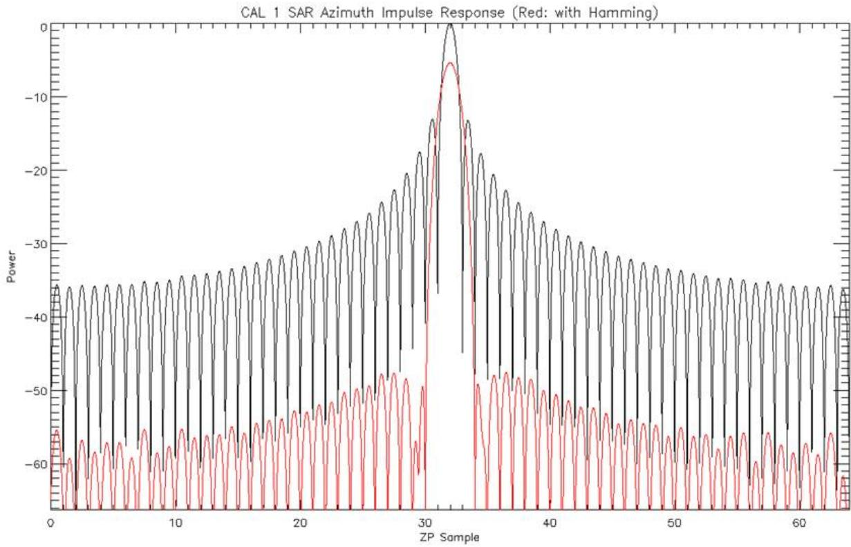
Figure 10: Comparison of AIR with and without Hamming window (full range)
