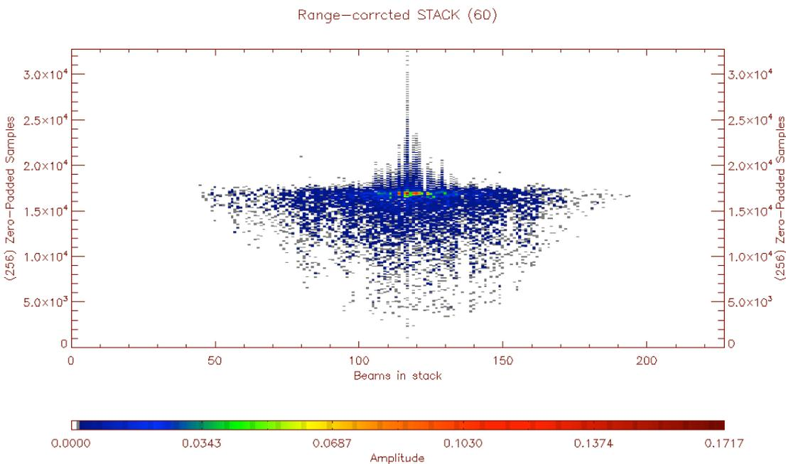
Figure 15: Stack 60 with hamming: the nadir clutter has disappeared
