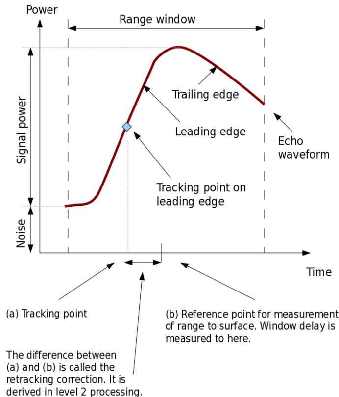
**Figure 16: Idealised pulse-limited waveform in window**
