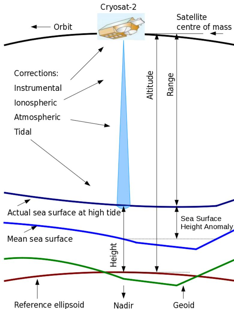
Figure 7: Basic altimetry terms and applicable corrections over open ocean
