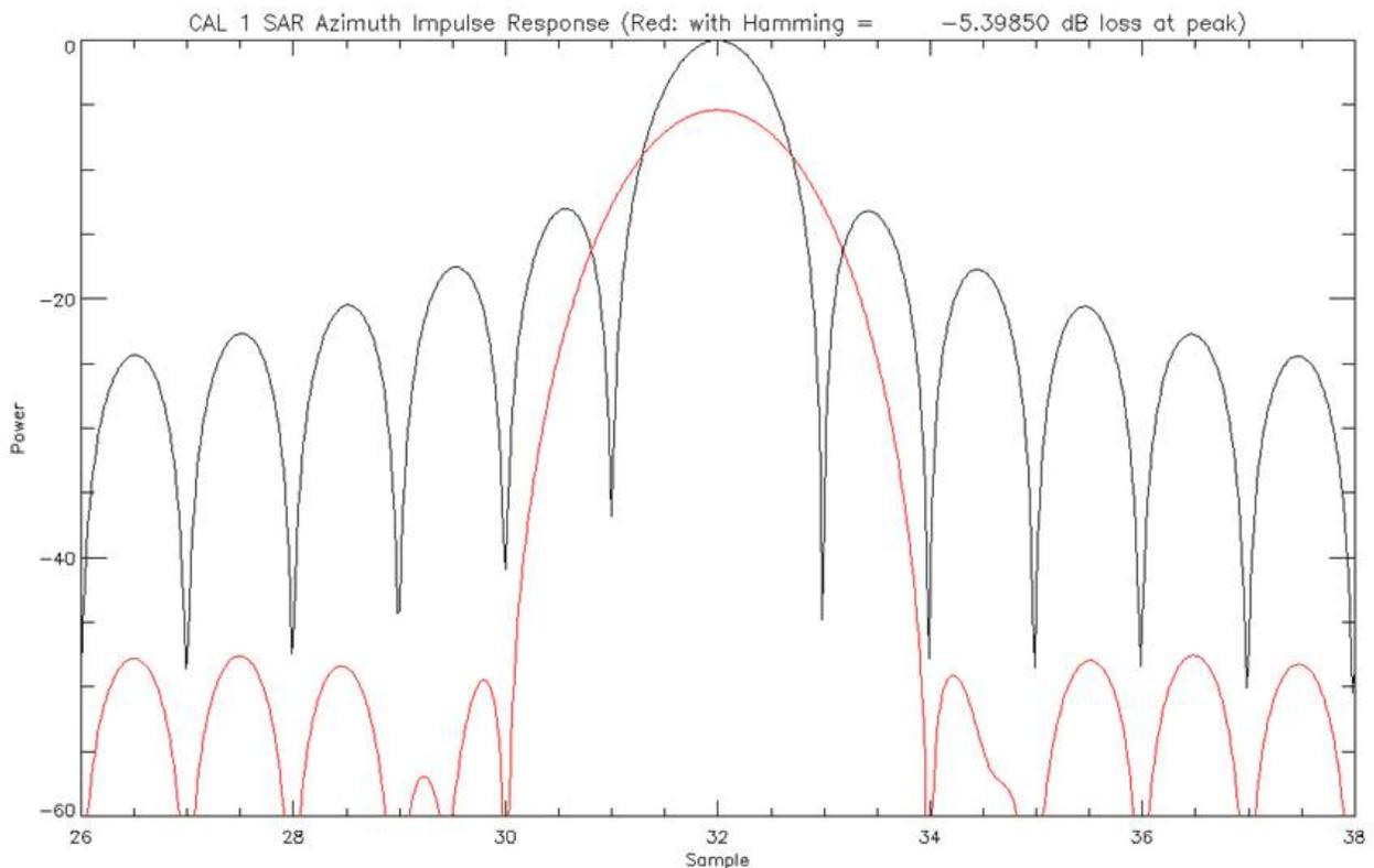
Figure 9: Comparison of AIR with and without Hamming window
