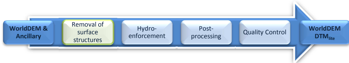
Figure 3-1: WorldDEM DTM lite main processing steps
