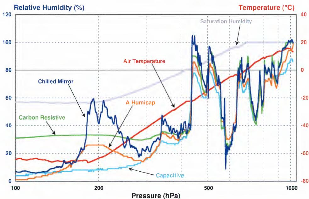
*Figure 2.6: Comparison between humidity soundings made at Wallops Island on 1 June, 1998 for four different sensors launched on the same balloon (courtesy: F. J. Schmidlin). Three of these sensors (A-humicap, carbon resistive and capacitive) have been or are currently routinely used by US or European weather services.*
