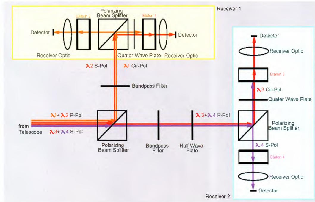
**Figure 6.11:** Receiver principle.
