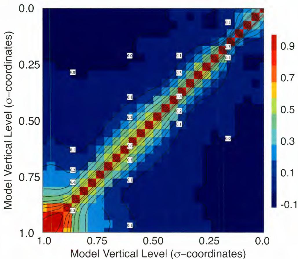
**Figure 2.5:** Background vertical error correlation matrix for the humidity variable used at the MSC. The bottom-left corner represents the surface-surface component and the upper-right corner the top-top component (at 10 hPa). There are 28 vertical levels.
