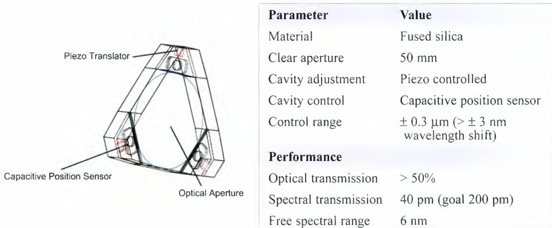
**Figure 6.12:** Etalon proposed design. **Table 6.4:** Etalon performance and design values.
