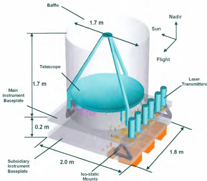
**Figure 6.13:** Instrument mechanical layout.
