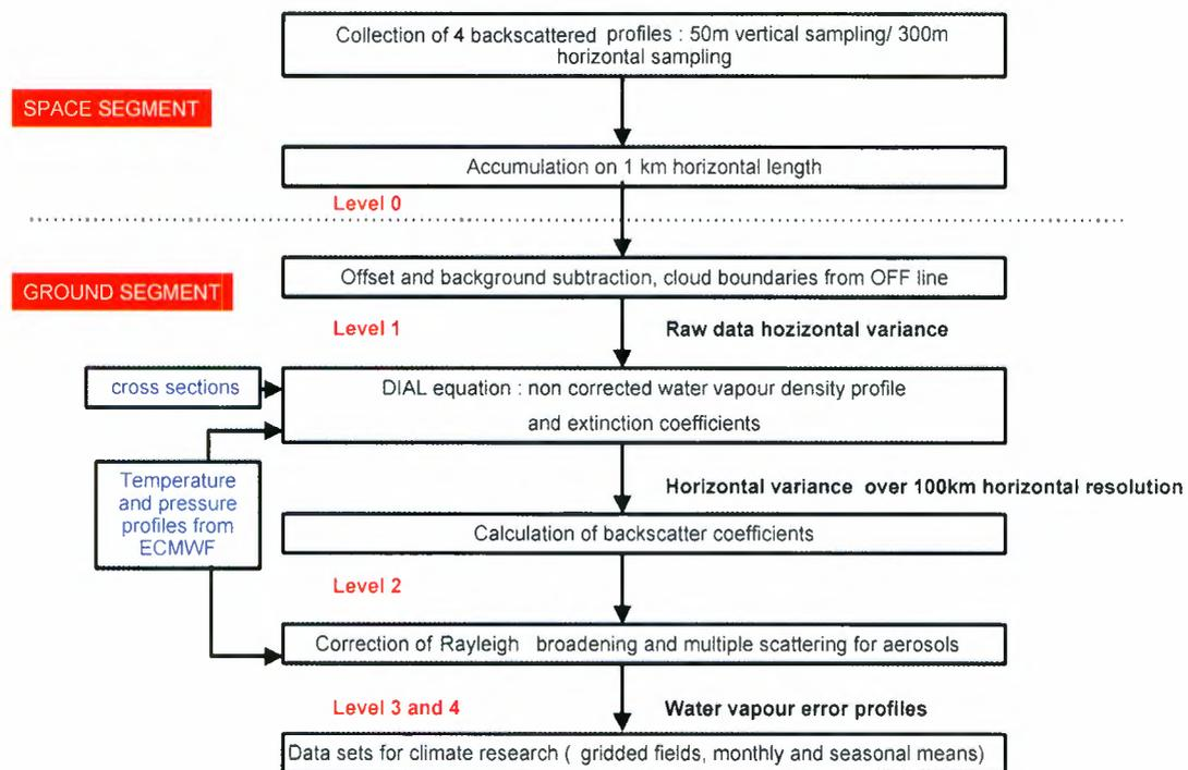
*Figure 6.20: Data processing flow diagram.*
