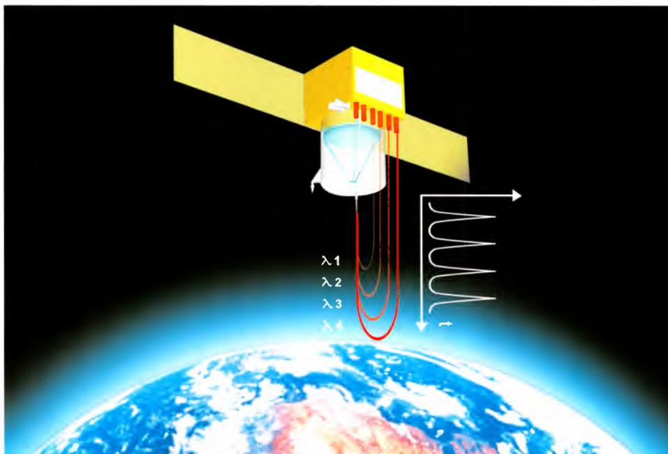
*Figure 6.1: Observational principle of WALES.*
