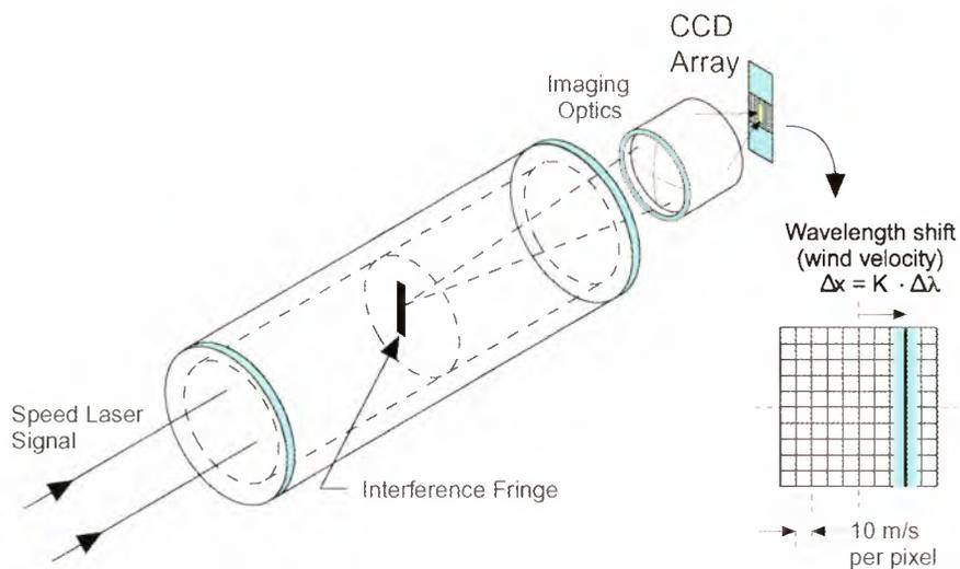
**Figure 6.8:** *Wavemeter principle.*
