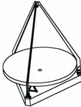
**Figure 6.9:** 1.5 m diameter telescope. All ceramic CSiC design.
