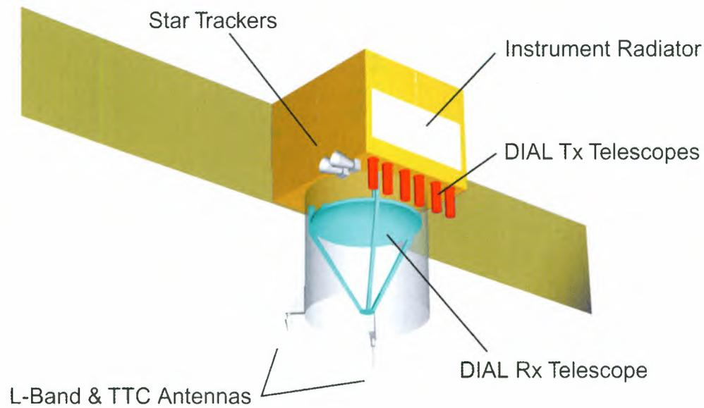
*Figure 6.16: Spacecraft in deployed configuration.*
