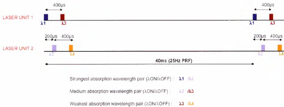
**Figure 6.4:** Operation principle and temporal diagram of emitted wavelengths. A train of pulses is emitted in burst mode at a 25 Hz pulse repetition rate. Pulses are emitted in a cascade with a delay of 200  $\mu$ s, allowing the on-line and off-line pairs to probe essentially the same volume.
