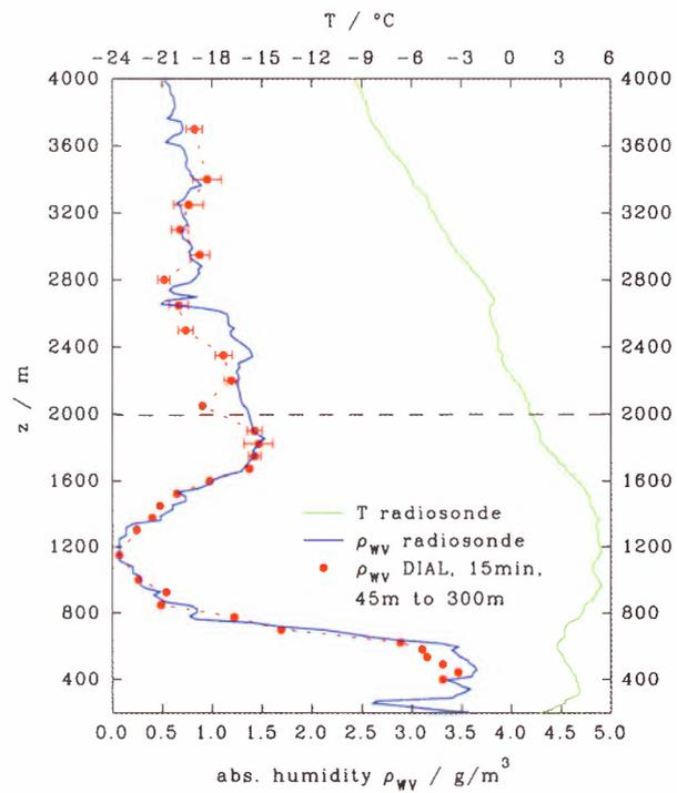
**Figure 5.3:** Water vapour and temperature profiles measured during the comparison experiment on 1 December 1994 at 19:13 UT. The DIAL profile was calculated without Doppler correction. Indicated in the DIAL profile are the statistical errors that are often less than the diameter of the circles. Excellent agreement between the water vapour profiles was achieved. Note the extended dry layer between 800 and 1400 m, which was very well captured by the DIAL.
