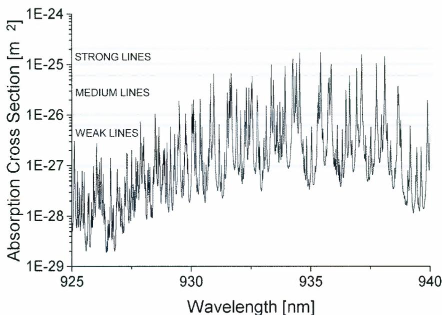
**Figure 5.2:** Water vapour absorption cross-section versus wavelength in the spectral region 925-940 nm. Horizontal lines highlight the cross-section ranges suitable for measurements in the upper, mid and low troposphere. Lines with strong absorption are suitable for sensing the upper troposphere/lowermost stratosphere (UTLS) region, medium absorption for the middle troposphere (MT) and weak absorption for the lower troposphere (LT).
