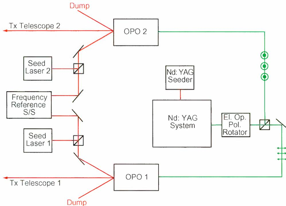
**Figure 6.6:** Principle of one transmitter unit.
