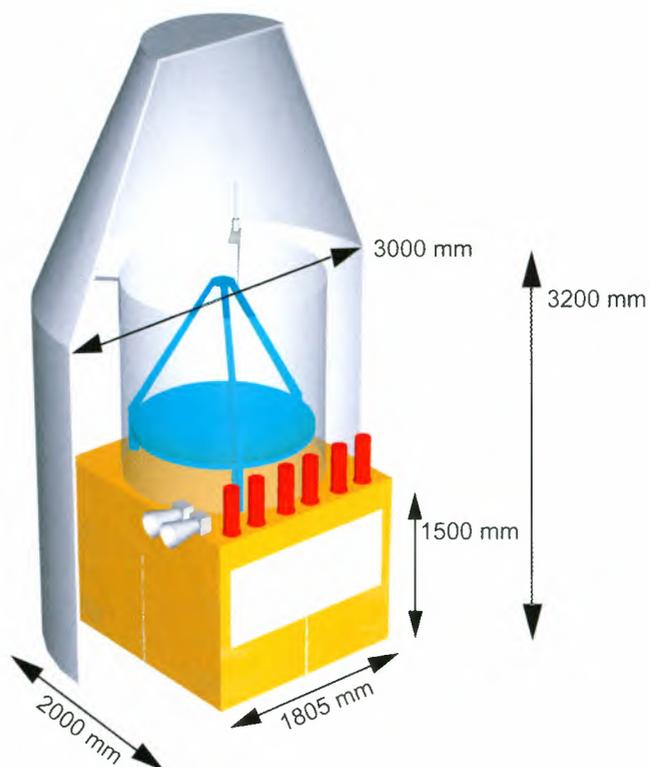
*Figure 6.18: Satellite stowed configuration in Soyuz IKAR launcher.*
