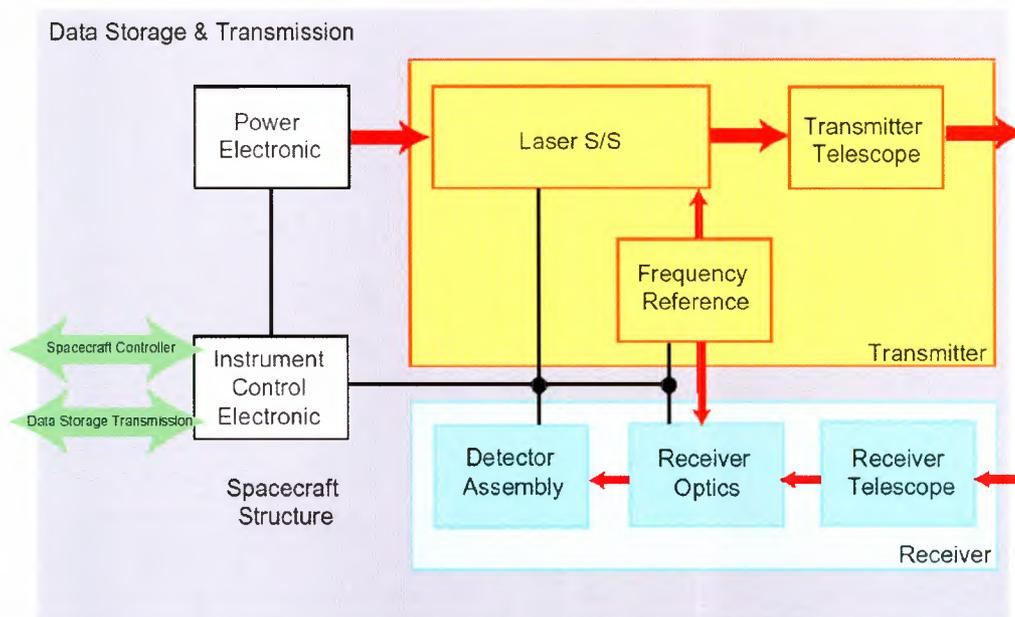
**Figure 6.5:** DIAL instrument functional block diagram.
