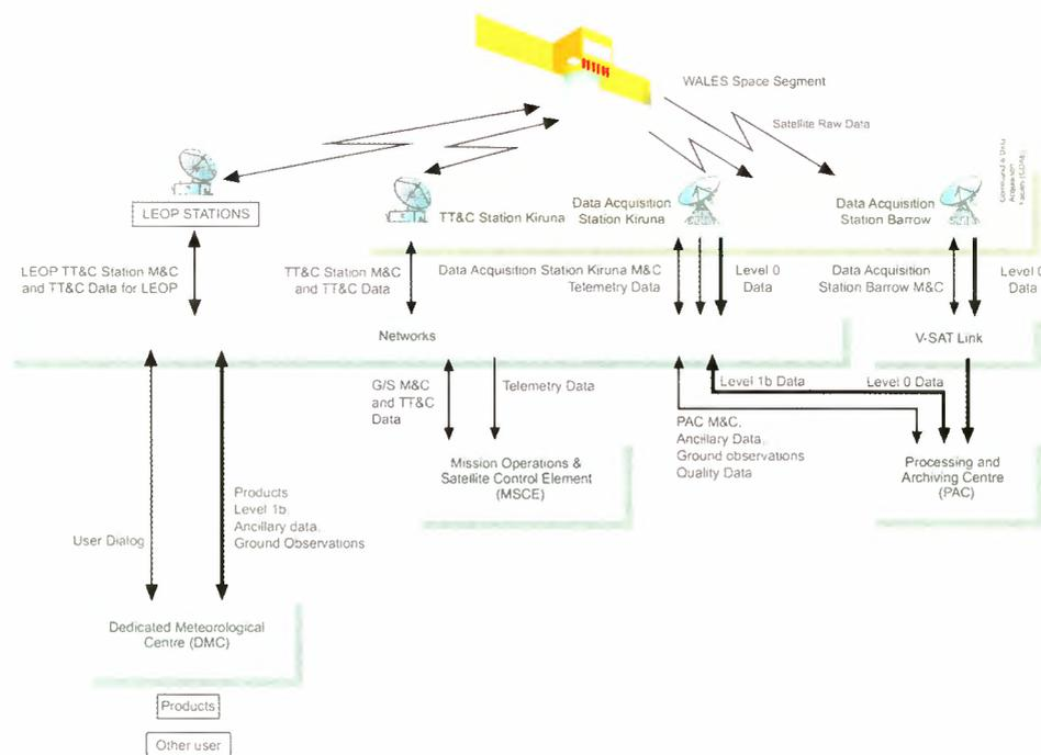
**Figure 6.19:** Ground segment architecture.
