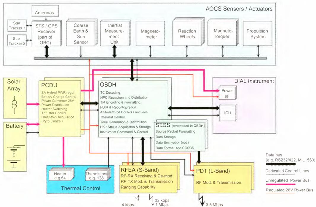
**Figure 6.17:** Satellite functional block diagram.
