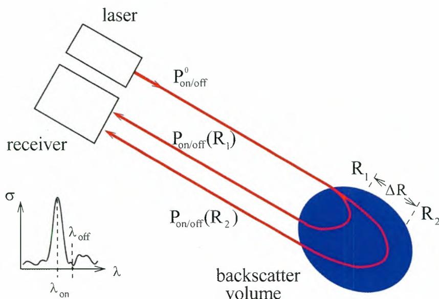
**Figure 5.1:** Conceptual drawing of the DIAL principle.
