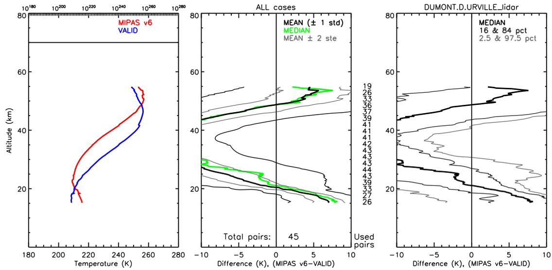
**Figure 3. Validation results using the Dumont d'Urville lidar. Engineering altitude grid is used. Plot composition as in Figure 2.**
