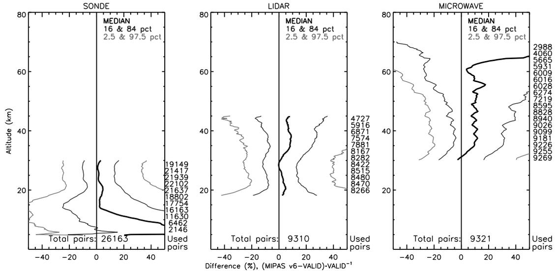
**Figure 6. Validation results for the MIPAS v6 ozone profiles compared to the three verification instruments: sonde (left), lidar (middle) and microwave radiometer (right) without application of the averaging kernels. Shown are the percentiles as before of the percent differences with respect to the verification instruments (MIPAS v6 - validation)/validation. Sonde data have been smoothed to a resolution of 3 km.**
