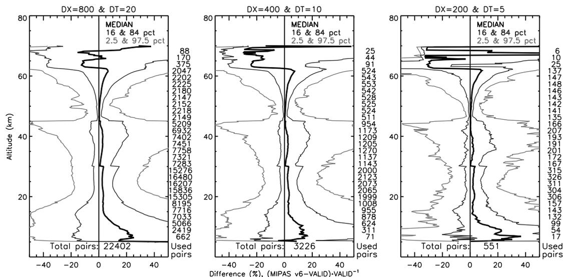
**Figure 10. Influence of collocation criteria on validation results. Left panel: max. 800 km and 20 hours (5 hours above 50 km) difference, middle panel: max. 400 km and 10 hours (5 hours above 50 km) difference, and right panel: max. 200 km and 5 hours difference.**
