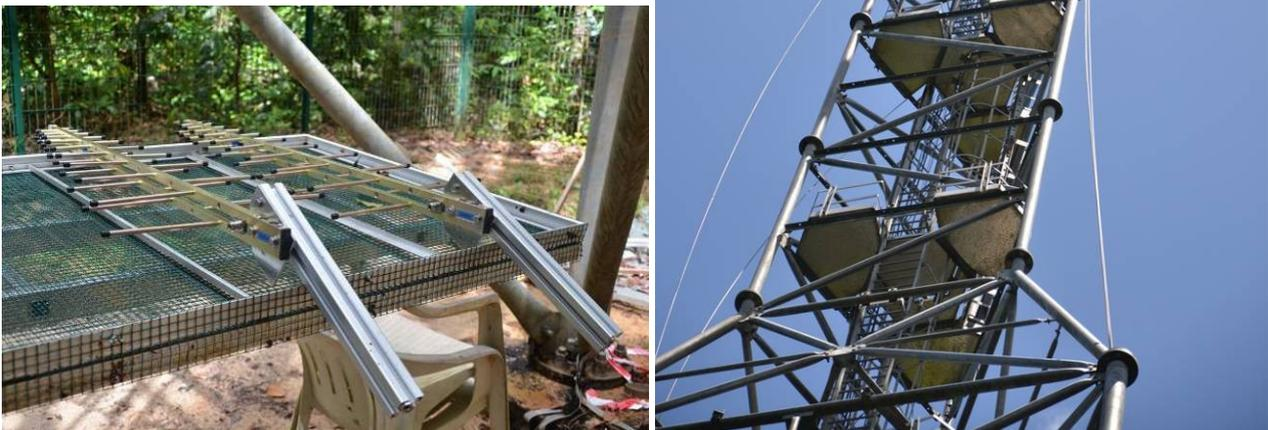
**Figure 5 - Set up of the antennas (left) on the tower, so as to form the vertical array (right)**
