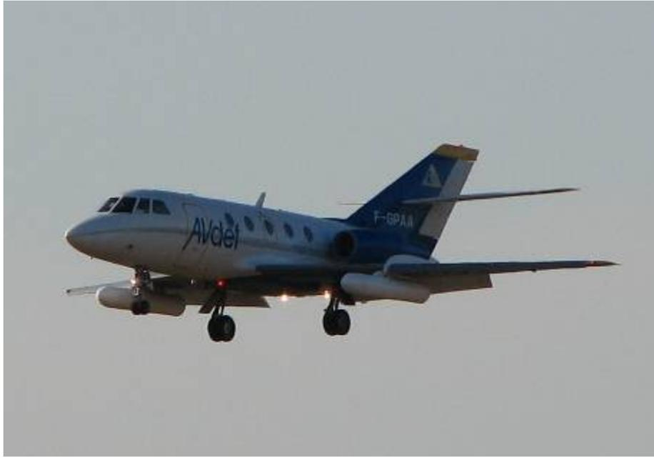
Figure 83: The Falcon 20 carrying the SETHI system. The two pods contain the radar antennas.
